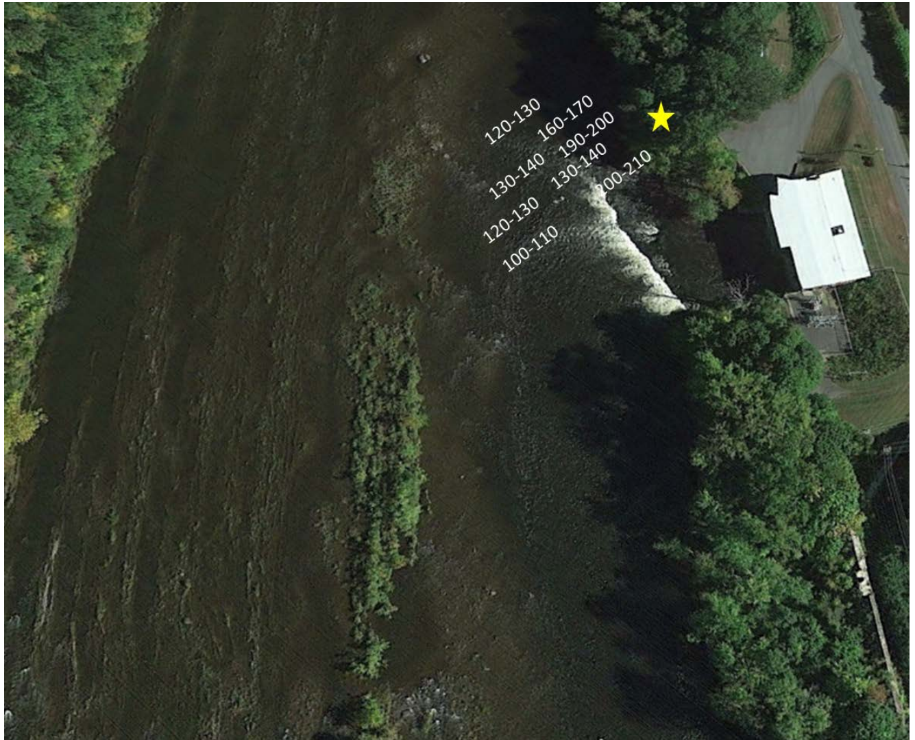
Figure 16: The yellow star marks the approximate placement of the 6-Element Yagi antenna and the Lotek receiver used to detect fish moving upstream through the Bypass Reach, downstream of Station 1. The radio test tag produced power levels ranging from 100 to 210 db with highest powers located near the yagi antenna and attenuating toward the opposite bank of the river.
