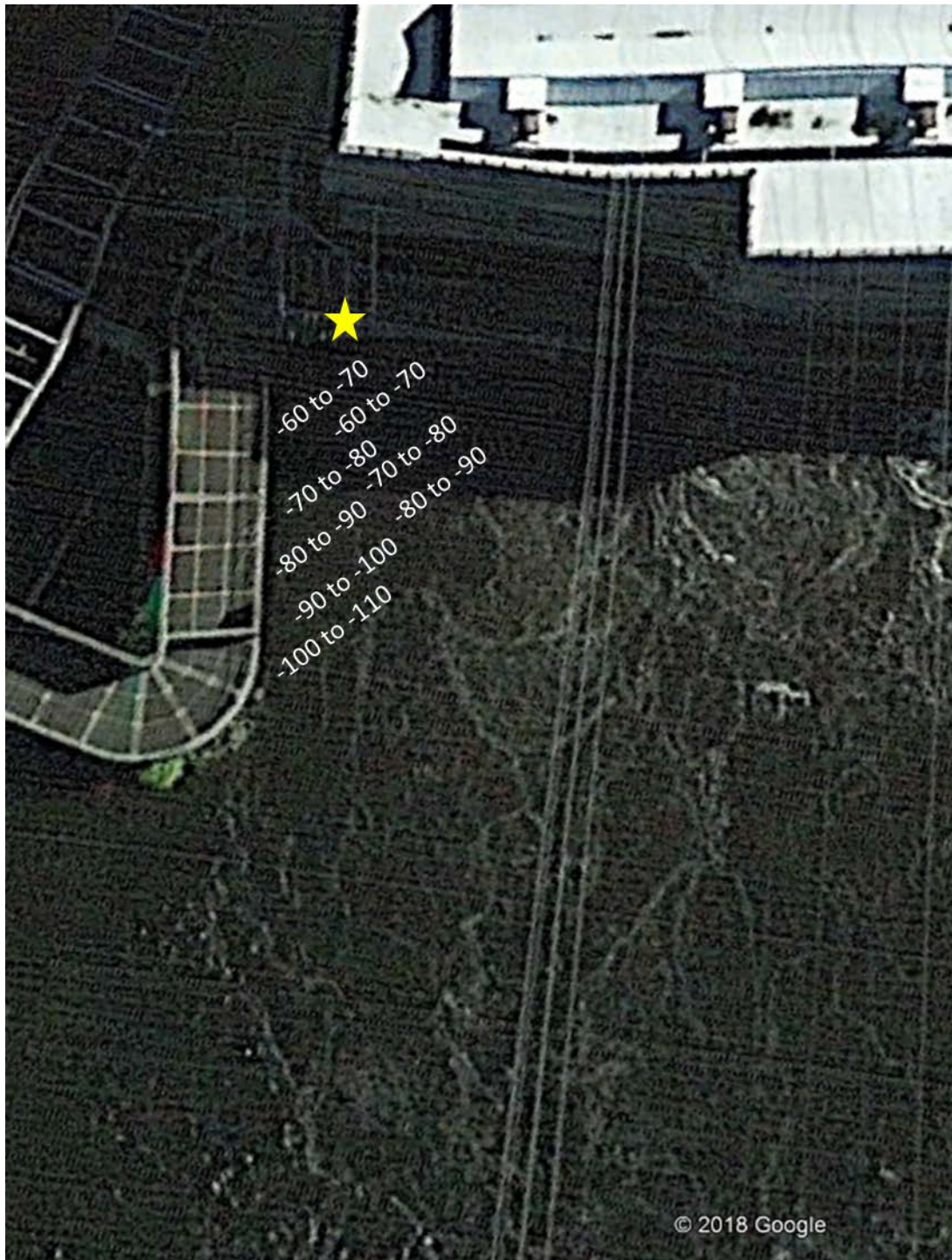
Figure 7: The yellow star marks the approximate placement of the dipole antenna and the Orion receiver used to detect fish moving to the Cabot Ladder entrance at River Mile 120. The radio test tag produced power levels ranging from -60s to -110s db with highest powers located near Cabot Fish ladder entrance and attenuating slightly farther out.
