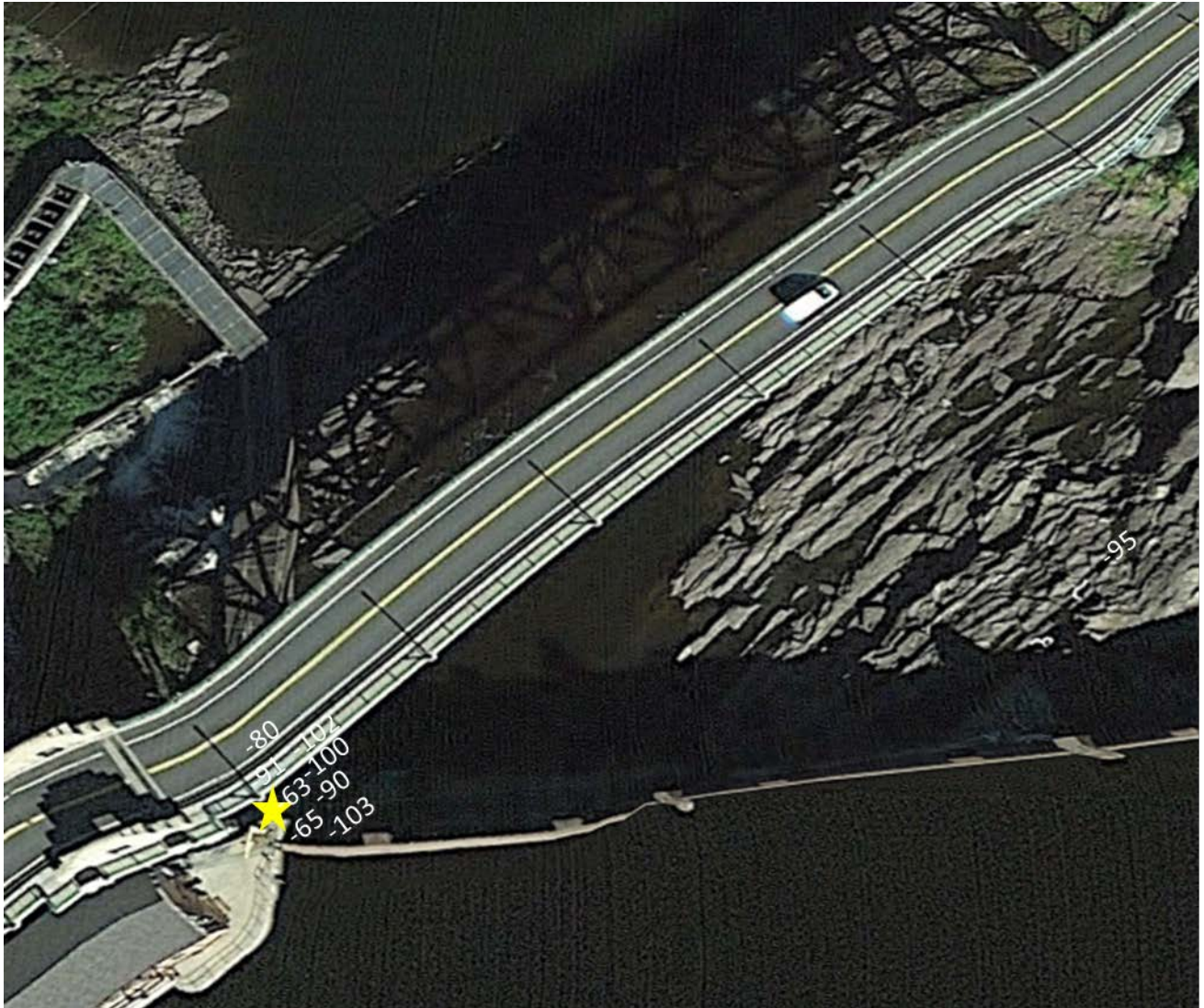
Figure 17: The yellow star marks the approximate placement of the dipole antenna and the Orion receiver used to detect fish moving upstream through the spillway fish ladder entrance. The radio test tag produced power levels ranging from -63 to -102 db with highest powers located near the dipole antenna and attenuating away from the dipole.
