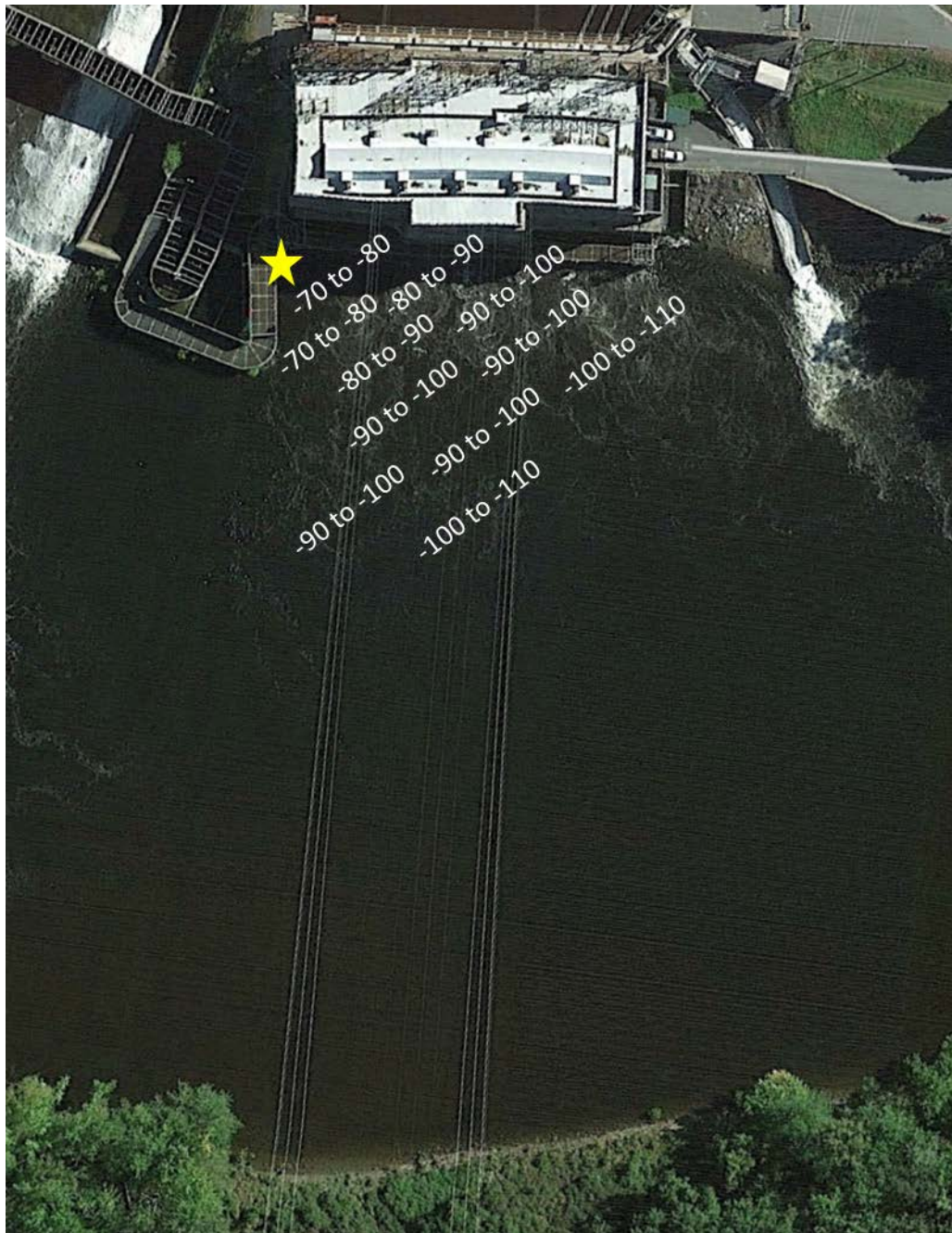
Figure 6: The yellow star marks the approximate placement of the yagi antenna and the Orion receiver used to detect fish moving in the Cabot Tailrace at River Mile 120. The radio test tag produced power levels ranging from -70s to -110 db at both locations with highest powers located closest to the yagi antennas and attenuating slightly toward the opposite bank.
