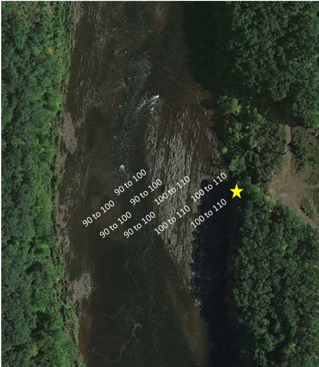
Figure 14: The yellow star marks the approximate placement of the 6-Element Yagi antenna and the Lotek receiver used to detect fish moving upstream through the Bypass Reach, upstream of Rawson Island. The radio test tag produced power levels ranging from 90s to 110 db with highest powers located near the yagi antenna and attenuating toward the opposite bank of the river.
