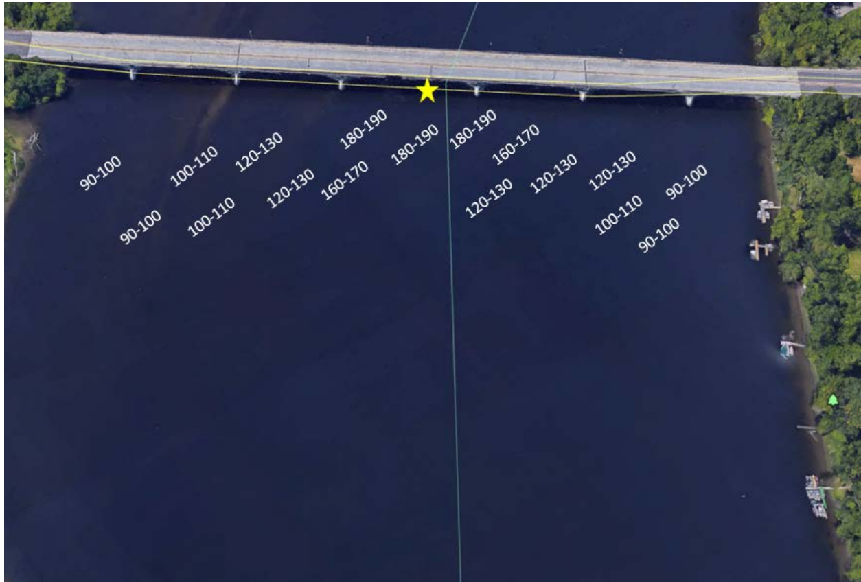
Figure 24: The yellow star marks the approximate placement of the yagi antenna and the Lotek receiver used to detect fish moving upstream towards Cabot station from the Rt.202 Bridge in Holyoke, MA. The radio test tag produced strong power levels ranging from 90 to 190 db near the antenna.
