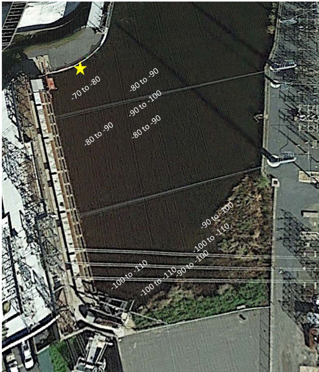
Figure 19: The yellow star marks the approximate placement of the yagi antenna and the orion receiver used to detect fish moving downstream towards the Cabot station forebay. The radio test tag produced power levels ranging from -70 to -110 db with highest powers located near the yagi antenna and attenuating toward the opposite bank of the river.
