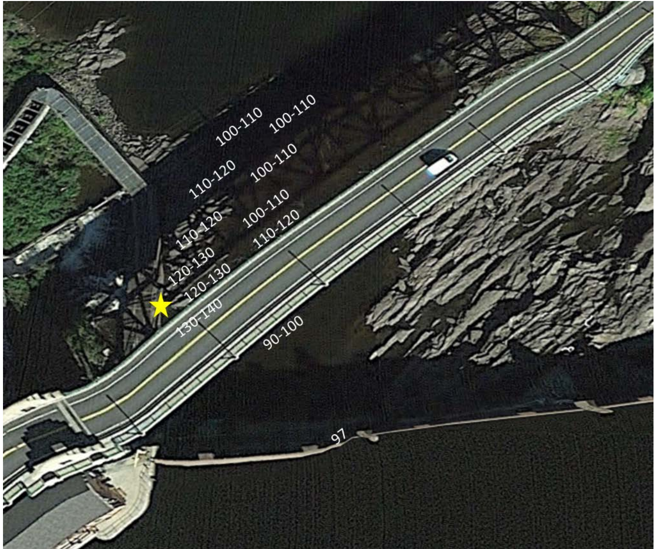
Figure 18: The yellow star marks the approximate placement of the yagi antenna and the Lotek receiver used to detect fish moving upstream towards the spillway fish ladder entrance. The radio test tag produced power levels ranging from 130 to 140 db with highest powers located near the yagi antenna and attenuating toward the opposite bank of the river.
