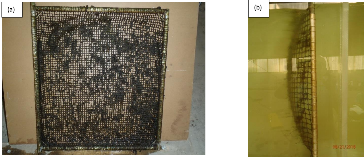
Figure 3-1. (a) The effect of bio-fouling on the sample net, (b) The test of the sample net panel in the lab flume.
