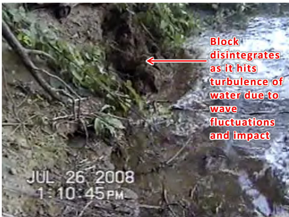
Figure 5.5.3-6b: Boat Wave Erosion Sequence
