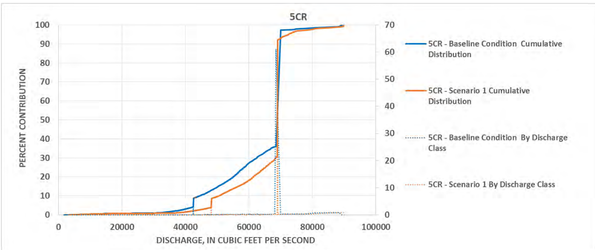
Figure 5.4.2.2-7 (Part 1 of 2): Distribution of Total Erosion at Four Sites According to Discharge Classes
