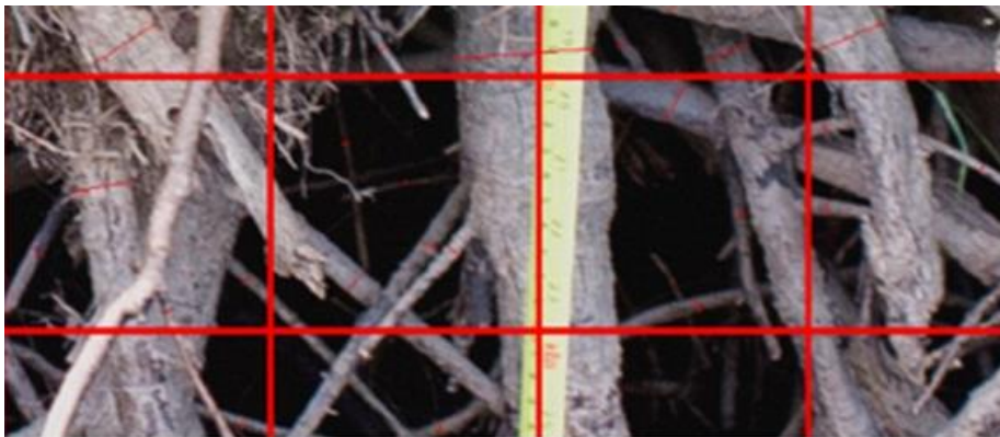
Figure 4.2.7.2-4: Zoomed Image with 0.1m x 0.1m Grid Superimposed, Showing Individual Root Diameter Measurements Made in SigmaScan
