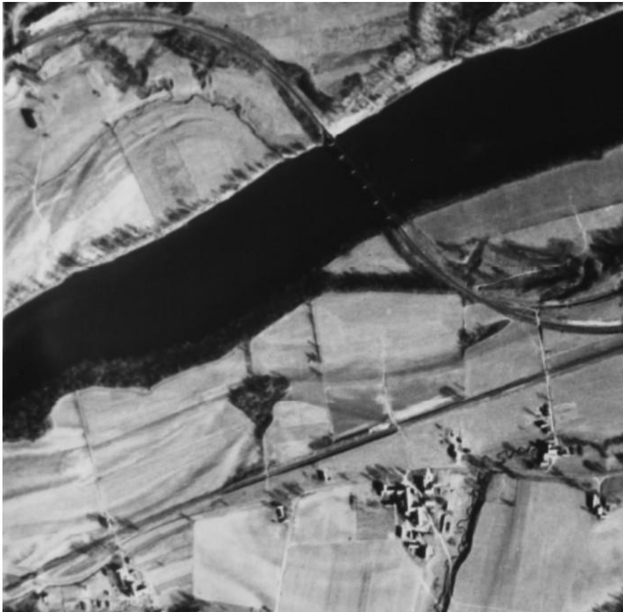
Figure 5.5.5.3 Aerial Photo Showing Erosion Scars on Floodplain - 1939
