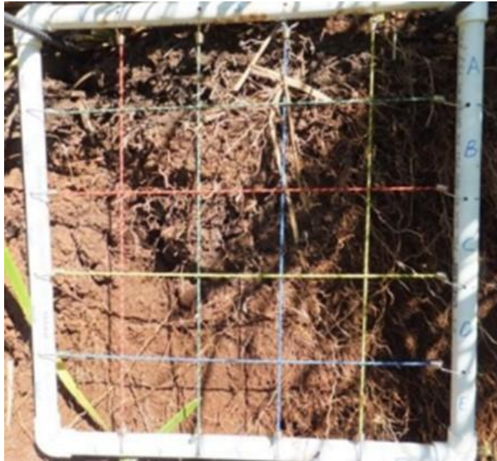
Figure 4.2.7.2-1: Example of Grid Used for Root Diameter and Density Measurements in the Field
