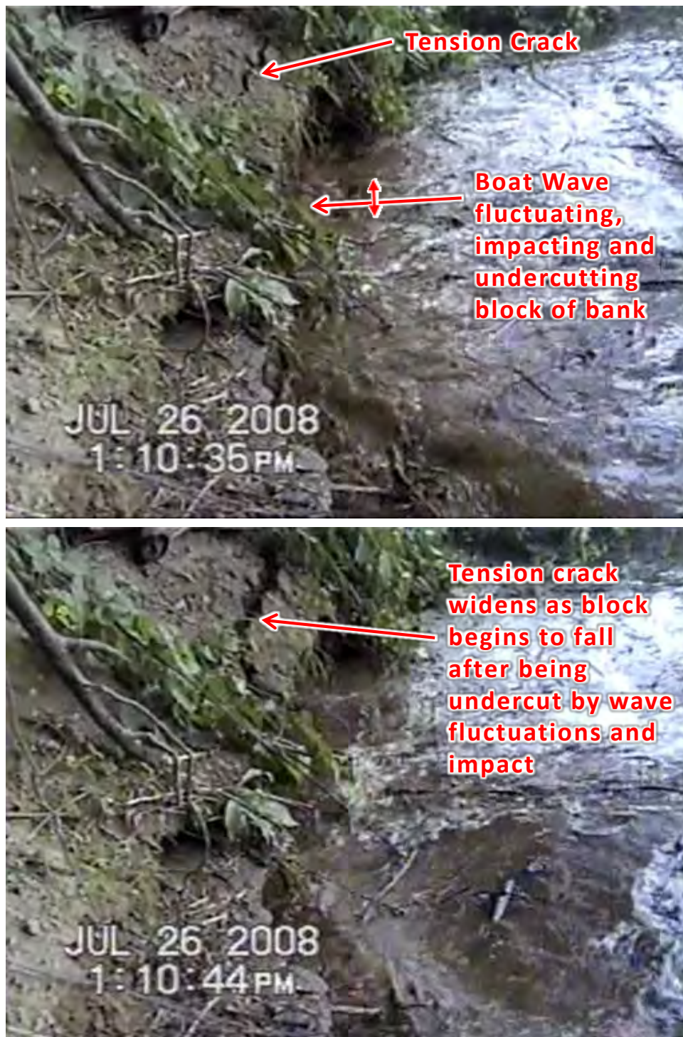
Figure 5.5.3-6a: Boat Wave Erosion Sequence
