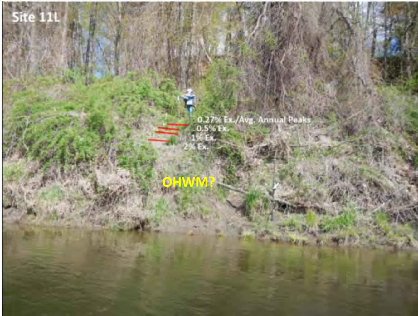
Figure 4.2.4.1-7 Physical characteristics of OHWM at Site 11L
