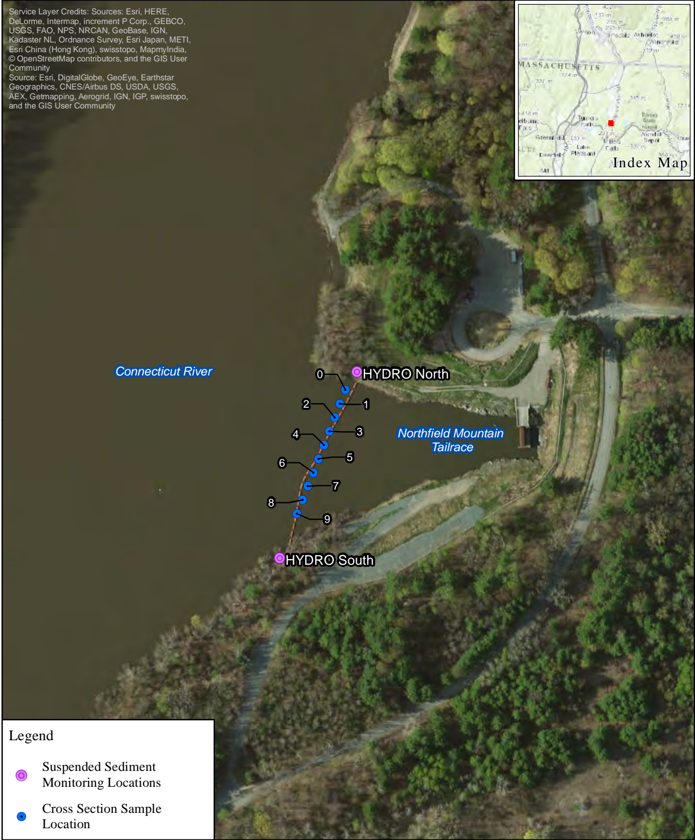
Figure 4.2.9-3: Location of LISST HYDROs and LISST-100X Cross-section
