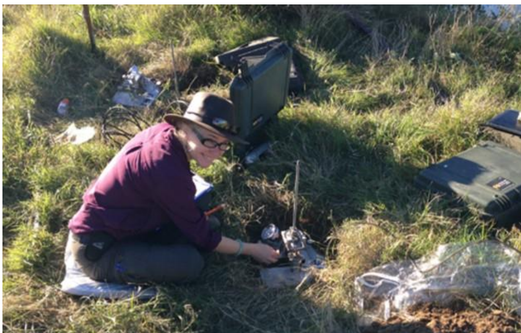
Figure 4.2.6.1-2: Conducting a Borehole Shear Test (BST)
