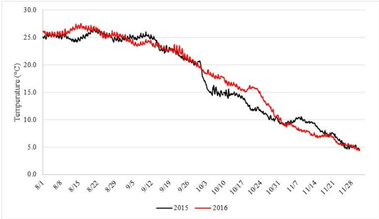
Figure 4.1.7-1. Water temperature (°C) as measured in the power canal Turners Falls, MA
