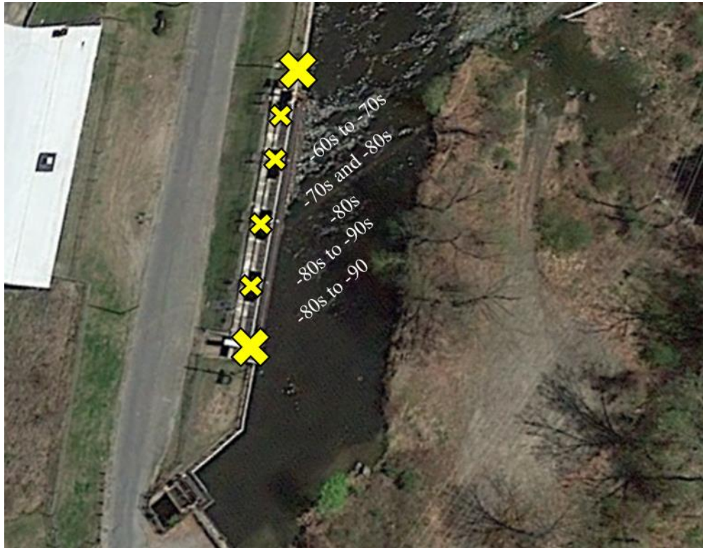
Figure A-5: The large X's mark the approximate placement of the Yagi antennas and Orion receivers used to detect fish within the vicinity of the Station No. 1 Forebay. Small X's mark the placement of four in-water droppers used to assist with monitoring eel passing through the intake. A radio test tag produced power levels ranging from -60 to -90 dB, with higher power levels closer to the Yagi antennas and slightly lower power levels toward the middle of the forebay.
