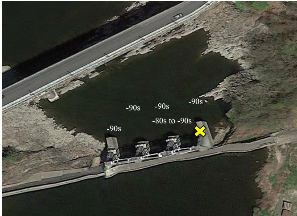
Figure A-8: The X marks the approximate placement of the Yagi antennas and Orion receiver used to detect fish below the Turners Falls Dam at River mile 122. The radio test tag produced power levels ranging from -80 to -90s dB, with highest power levels located closest to the Yagi antenna.
