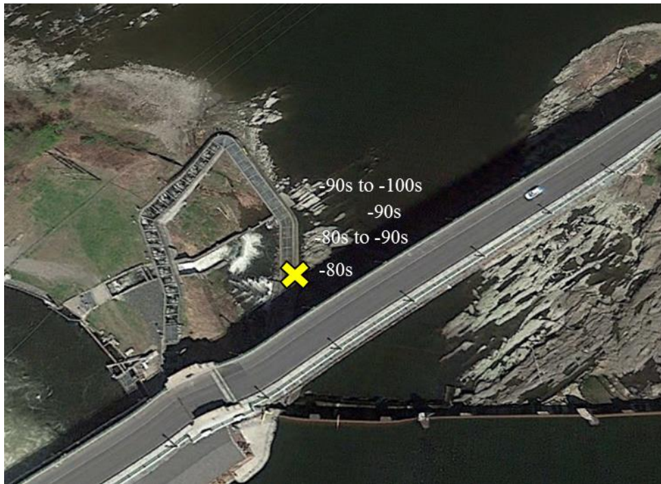
Figure A-6: The X marks the approximate placement of the Yagi antennas used, in conjunction with an Orion receiver, to detect fish within the vicinity of the fishway below the Turners Falls Dam, at River Mile 122. The radio test tag produced power levels ranging from -80 to -100s dB, with higher power levels closer to the Yagi antenna.
