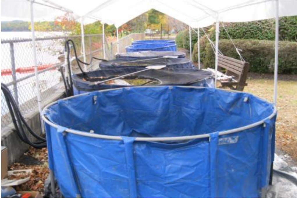
Figure 4-7: On shore eel holding tanks (900 gal) to monitor delayed effects of tagging and turbine passage. Tanks continuously supplied with ambient river water by two redundant pump systems connected to different electrical circuits.
