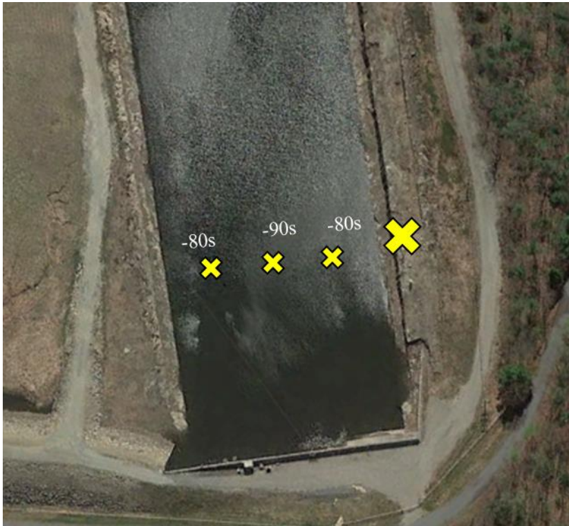
Figure A-14: The large X marks the approximate placement of the Yagi antenna and Orion receiver used to detect fish in the Northfield Mountain Upper Reservoir intake/discharge. Small X's mark the approximate placement of three in-water droppers used at this location to assist with monitoring the passage of downstream eel. The radio tag was tested at a depth of approximately 5 ft. Power levels remained consistent across the intake ranging from -80 to -90s db. Some noise was detected at this site, and amplification was used with the Orion receiver.
