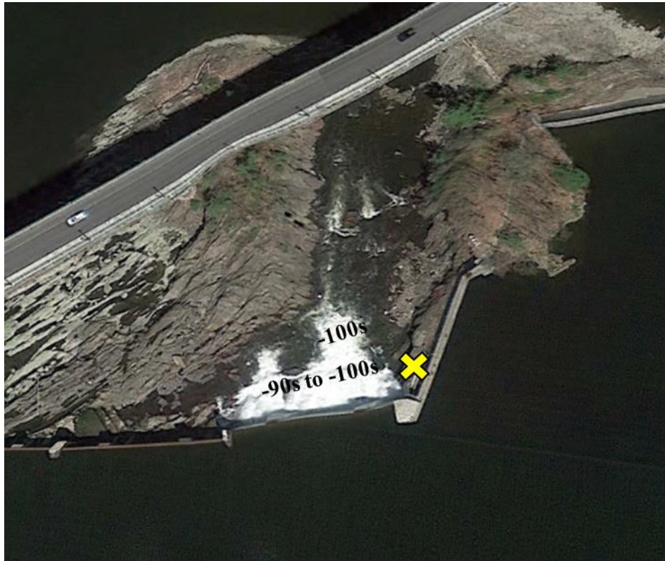
Figure A-7: The X marks the approximate placement of the Yagi antennas used, in conjunction with an Orion receiver, to detect fish below Bascule Gate 4. The radio test tag produced power levels ranging from -90 to -100s db.
