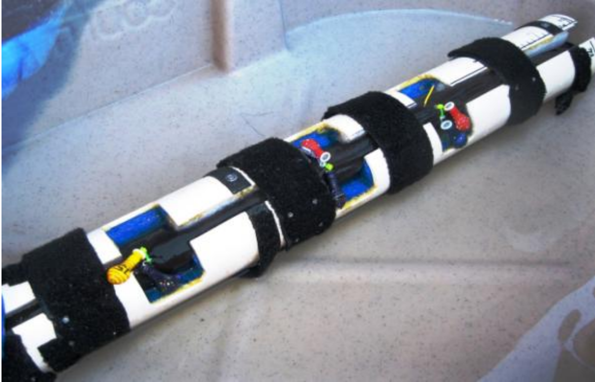
Figure 4-2: Specially designed eel restraining device used to aid in HI-Z tagging adult American Eels.
