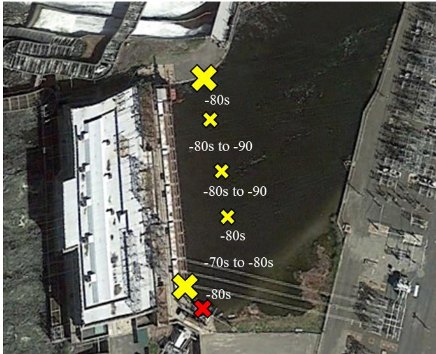
Figure A-4: The large Yellow X's mark the approximate placement of the Yagi antennas and Orion receivers used to detect fish within the vicinity of the Cabot Station forebay. Small yellow X's mark the approximate placement of three in-water droppers used to assist with monitoring the passage of downstream eel nearer to the intake grates. A radio tag was tested at a depth of approximately 2.5ft. Power levels remained strong across the forebay ranging from -70 to -90 db. The small red X marked the location of a dipole antenna and Orion receiver used to monitor eel moving through the downstream bypass. The test tag was read within a 20ft radius with power levels in the -80s db.
