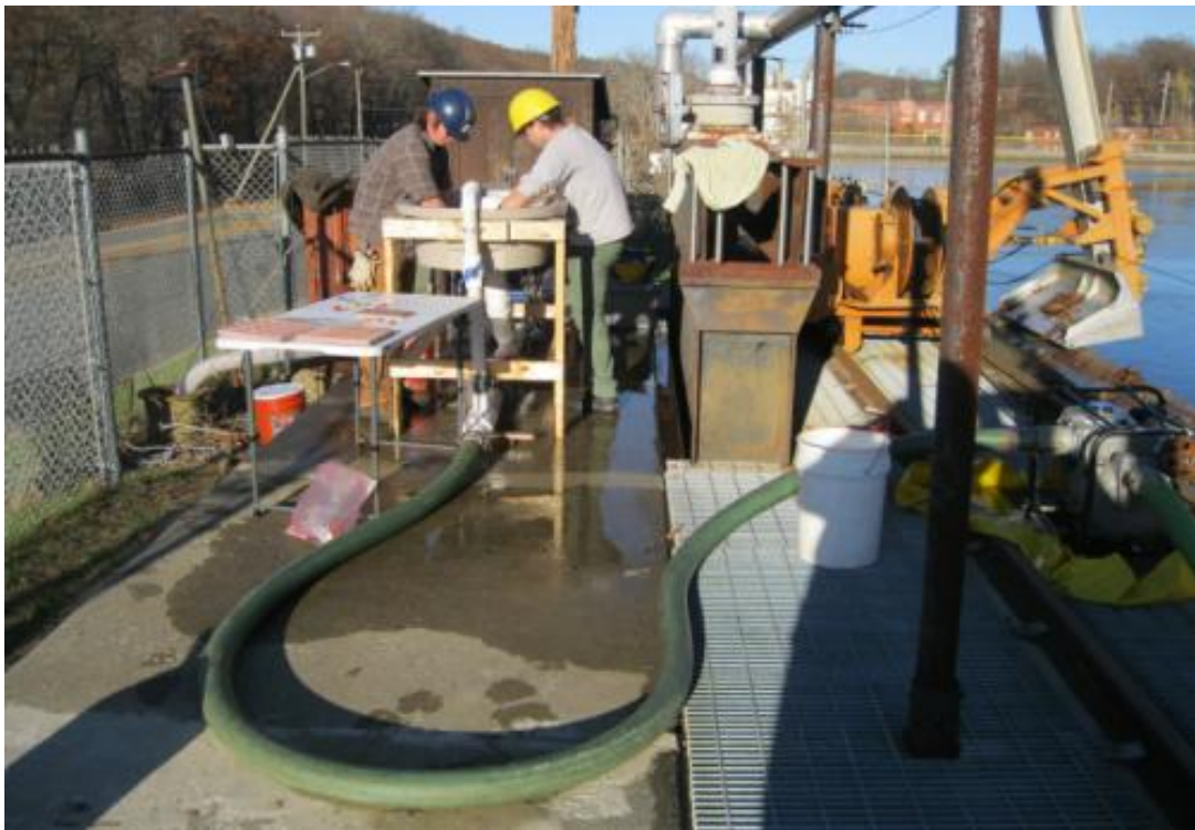
Figure 4-4: Adult eels released through an induction apparatus. The induction system and release hose supplied with river water by a 3-inch trash pump that transported eels quickly to the desired release point.
