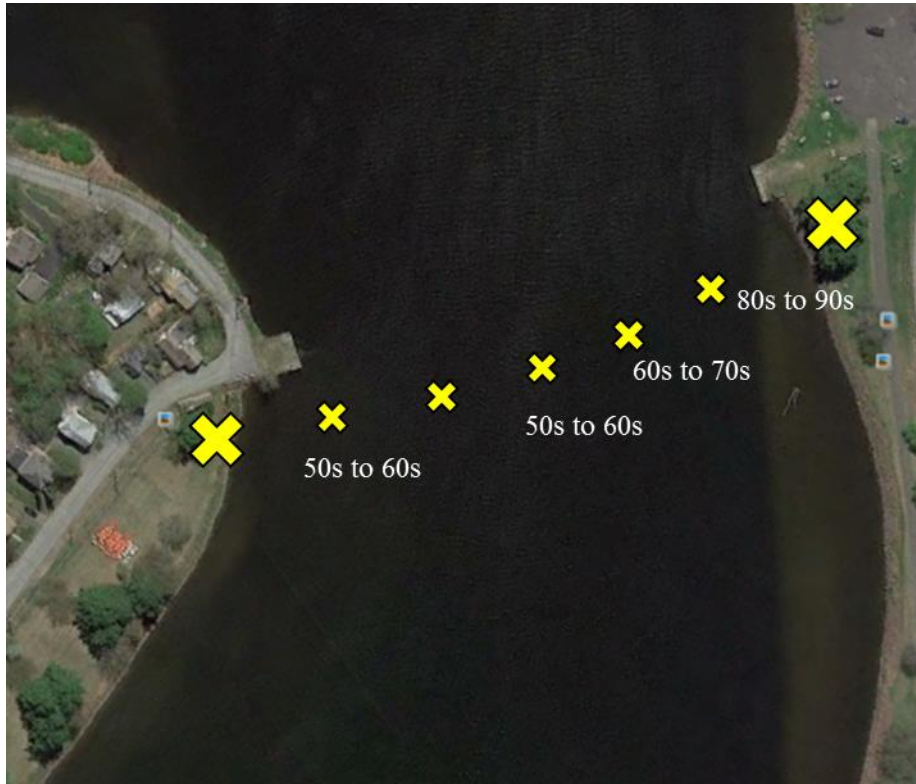
Figure A-11: The large X marks the approximate placement of each Yagi antenna and the Lotek SRX receiver used to detect fish across the width of the river, upstream of Turners Falls Dam. Small X's mark the approximate placement of five in-water droppers used at this location to assist with monitoring the passage of downstream eel. Power levels between the droppers ranged from 50s to 90s, with the test tag at 15 ft. A small area in the middle of the river had no detections with the tag at 15 ft, but registered at 5ft with a power level ranging from 60s to 70s.
