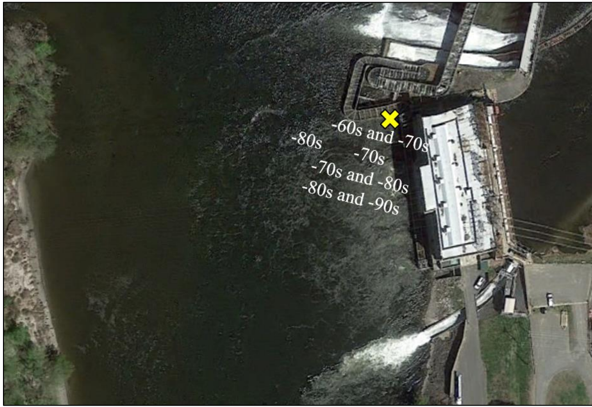
Figure 6: The large yellow X marks the approximate placement of the yagi antenna and the Orion receiver used to detect fish moving in the Cabot Tailrace at River Mile 120. The radio test tag produced power levels ranging from -60s to -90s db with highest powers located near Cabot Station Fish ladder closest to the yagi antenna and attenuating slightly farther out.
