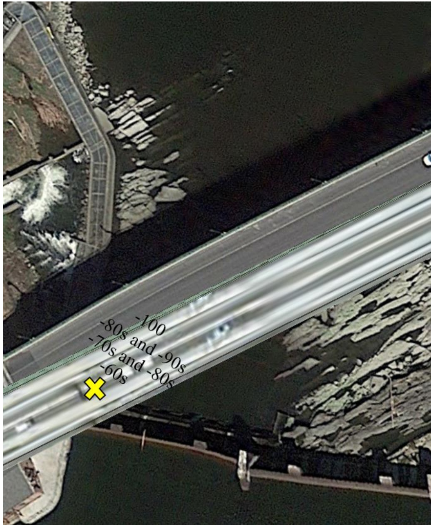
Figure 10: The large yellow X marks the approximate placement of the dipole antenna and the Orion receiver (under bridge) used to detect fish moving to the Spillway Ladder entrance at River Mile 120. The radio test tag produced power levels ranging from -60s to -100 db with highest powers located near Spillway Fish ladder entrance and attenuating farther out.
