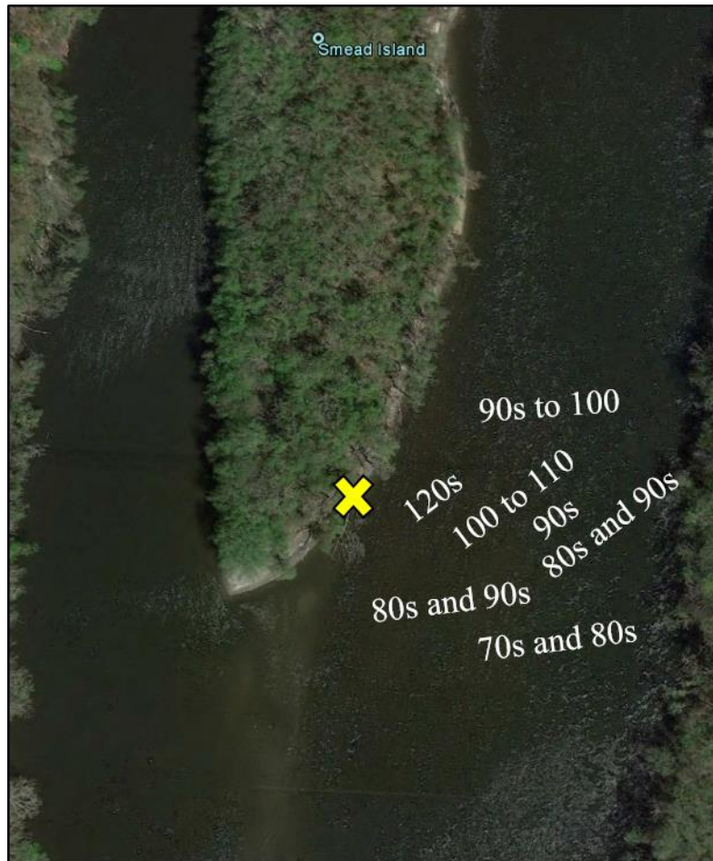
Figure 3: The large yellow X marks the approximate placement of the yagi antenna and the Lotek receiver used to detect fish moving across the width of the river at River Mile 120. The radio test tag produced power levels ranging from 70s to 120 db with highest powers located near the bank of the river on the East channel of Smead Island closest to the yagi antenna and attenuating slightly toward the far bank.
