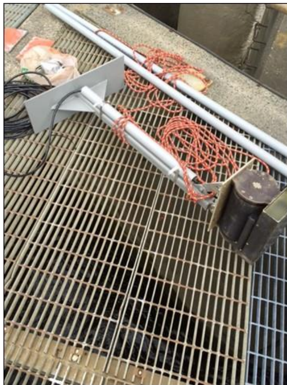
Figure 3.1.2-2: Pre installation of DIDSON camera mounted on custom fabricated bracket
