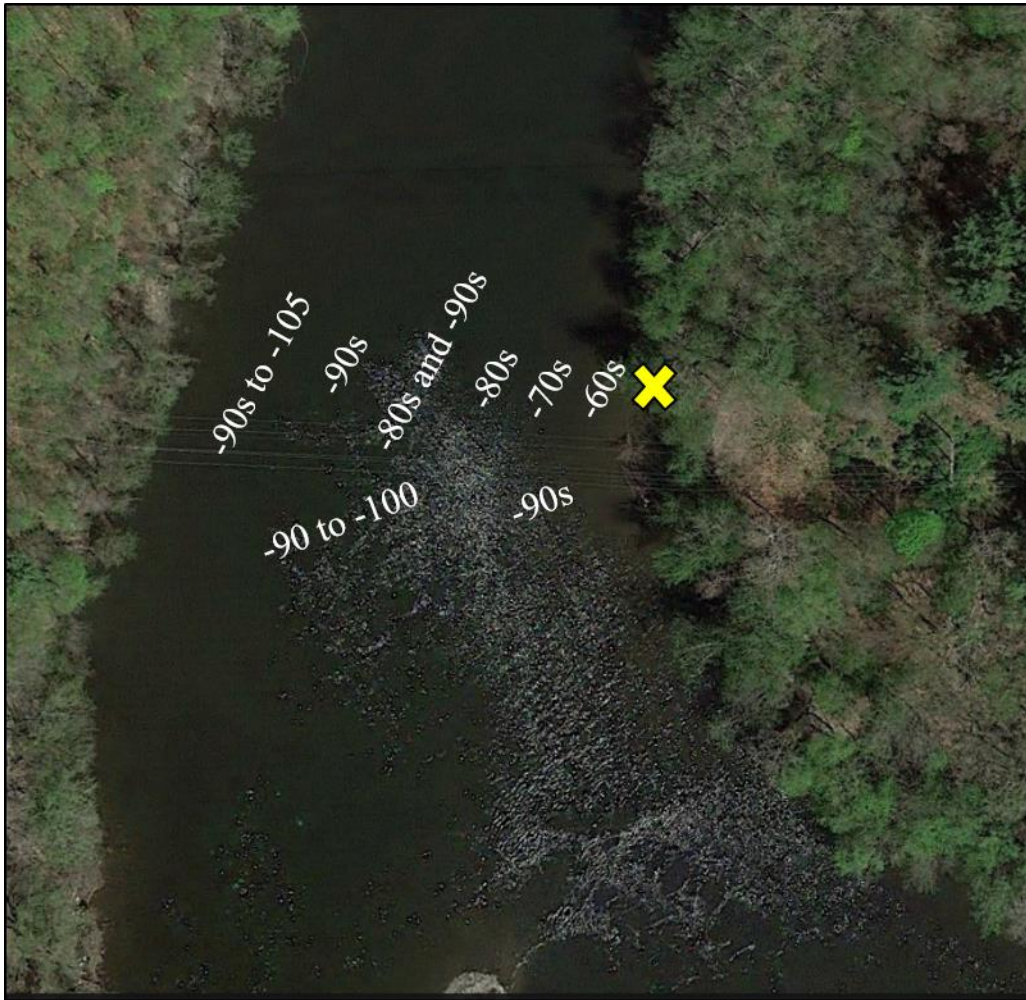
Figure 9: The large yellow X marks the approximate placement of the Yagi antenna and the Orion receiver used to detect fish moving upstream through to the Bypass Reach at River Mile 120. The radio test tag produced power levels ranging from -60s to -105 db with highest powers located near the yagi antenna and attenuating toward the opposite bank of the river.
