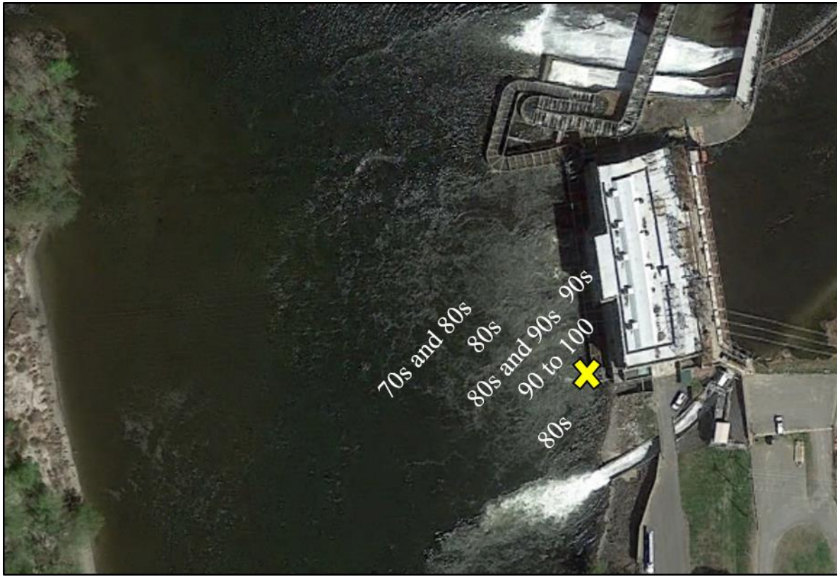
Figure 5: The large yellow X marks the approximate placement of the yagi antenna and the Lotek receiver used to detect fish moving into the Cabot Tailrace at River Mile 120. The radio test tag produced power levels ranging from 70s to 100 db with highest powers located near Cabot Station on the downstream end of the tailrace closest to the yagi antenna and attenuating slightly toward the far bank.
