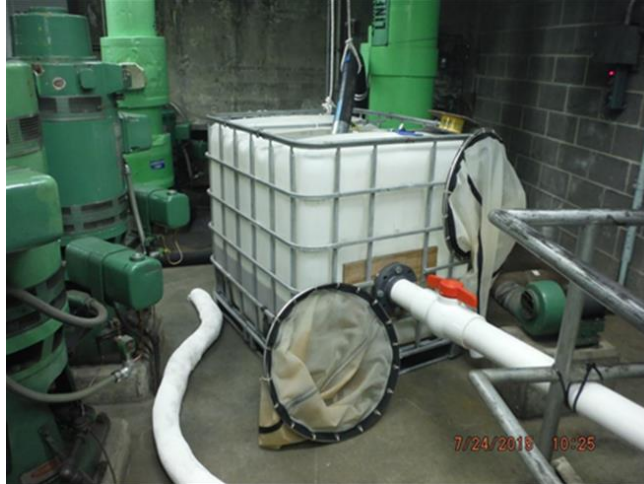
Figure 3.1-1: Ichthyoplankton Entrainment Sampling System for Collection of American Shad Eggs and Larvae at the Northfield Mountain Project.
