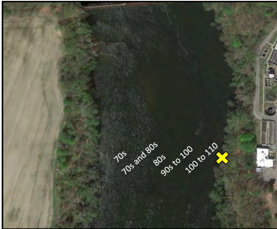
Figure 3: The large yellow X marks the approximate placement of the yagi antenna and the Lotek receiver used to detect fish moving across the width of the river at River Mile 119.5. The radio test tag produced power levels ranging from 70s to 110 db with highest powers located near the bank of the river closest to the yagi antennas and attenuating slightly toward the far bank.
