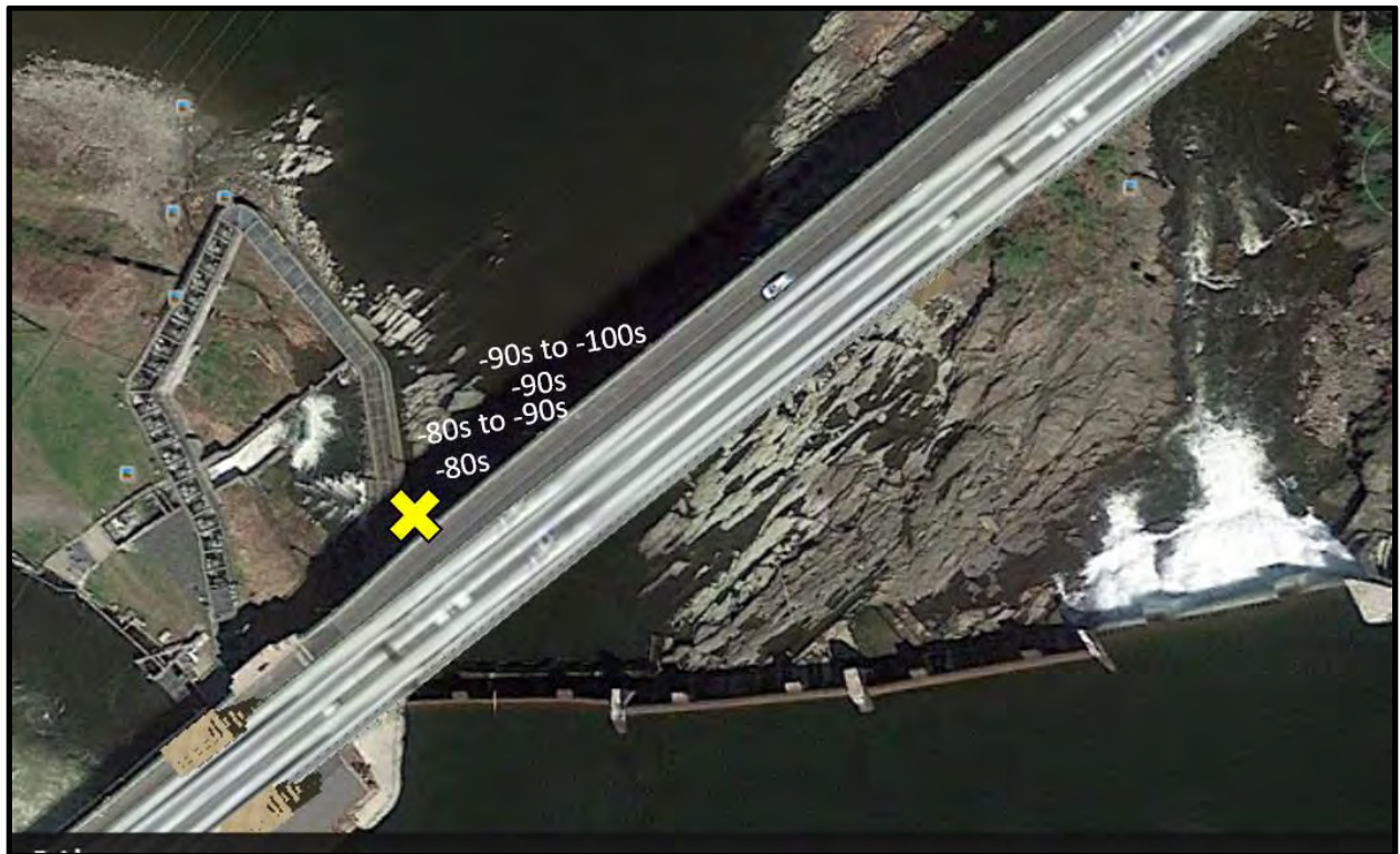
Figure 11: The large yellow X marks the approximate placement of the yagi antenna and the Orion receiver used to detect fish below the Turners Falls dam at River Mile 122. The radio test tag produced power levels ranging from -80 to -100s with highest powers located closest to the yagi antennas and attenuated farther out from the antenna. Not shown in this photo is a dipole antenna that was located at the entrance to the Spillway fish ladder. This antenna produced strong power levels ranging from -70 to -90.
