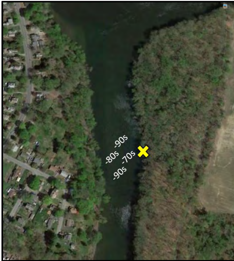
Figure 4: The large yellow X marks the approximate placement of the yagi antenna and the Orion receiver used to detect fish moving across the Deerfield River confluence at River Mile 119.5. The radio test tag produced power levels ranging from -70s to -90s db with highest powers located closest to the yagi antennas near Cabot Station and attenuating slightly further out in the tail waters.
