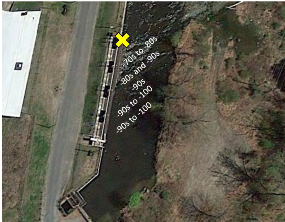
Figure 9: The large yellow X marks the approximate placement of the yagi antenna and the Lotek receiver used to detect fish within the Station No.1 tailrace at River Mile 121. The radio test tag produced power levels ranging from -70 to -90 with highest powers located closest to the yagi antennas and attenuated in the middle of the Cabot Station Forebay.
