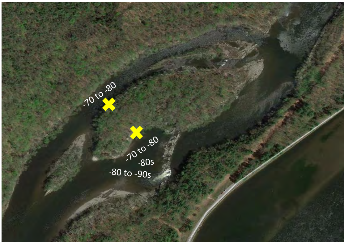
Figure 8: The large yellow X's mark the approximate placement of the yagi antennas and the Orion receivers used to detect fish moving across either side of Rawson Island at River Mile 120.5. The radio test tag produced power levels ranging from -70s to -90s with highest powers located closest to the yagi antennas and attenuated in the toward the far bank of the river.
