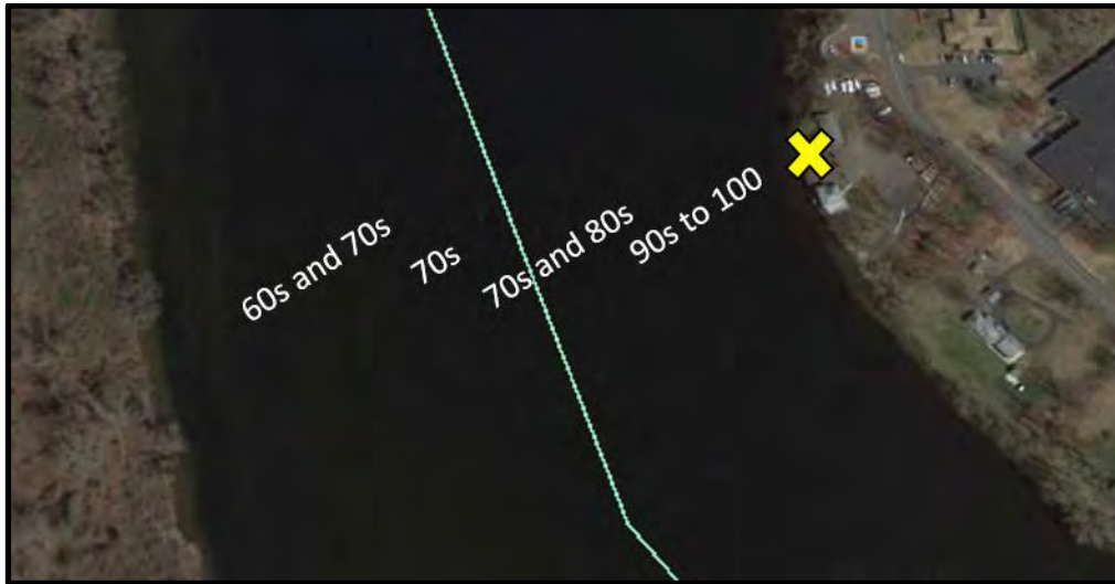
Figure 1: The large yellow X marks the approximate placement of the yagi antenna and the Lotek receiver used to detect fish moving across the width of the river at River Mile 86.5. The radio test tag produced power levels ranging from 60s to 100 db with highest powers located near the bank and attenuating slightly toward the far bank of the river.
