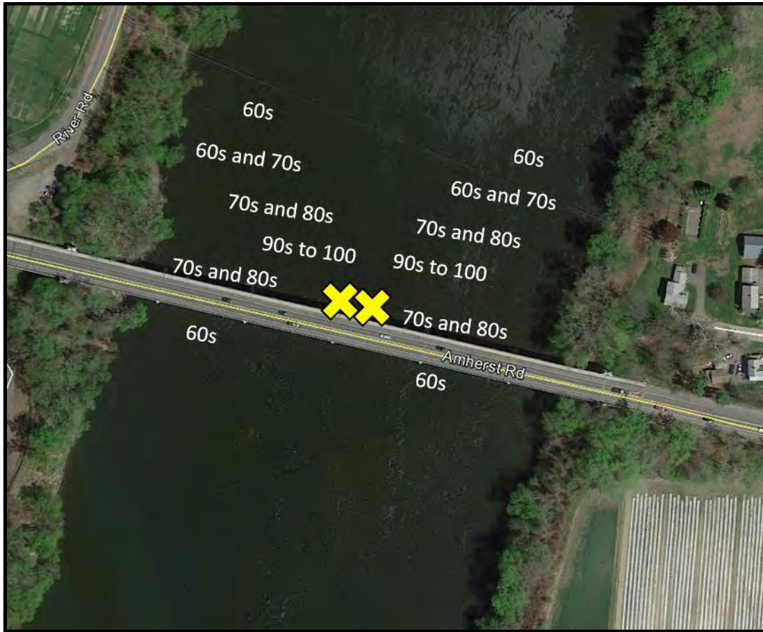
Figure 2: The large yellow X marks the approximate placement of the two yagi antennas and the Lotek receiver used to detect fish moving across the width of the river at River Mile 111. The radio test tag produced power levels ranging from 60s to 100 db with highest powers located near the middle of the river closest to the yagi antennas and attenuating slightly farthest from the approximate 45° angle of the detection zones.
