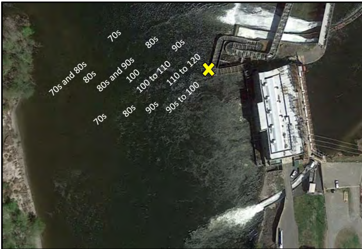
Figure 6: The large yellow X marks the approximate placement of the yagi antenna and the Lotek receiver used to detect fish moving across the width of the river passing Cabot Station at River Mile 120. The radio test tag produced power levels ranging from 70 to 120 db with highest powers located closest to the yagi antenna near the first bend in the Cabot Station Fish Ladder and attenuating toward the far bank of the river.
