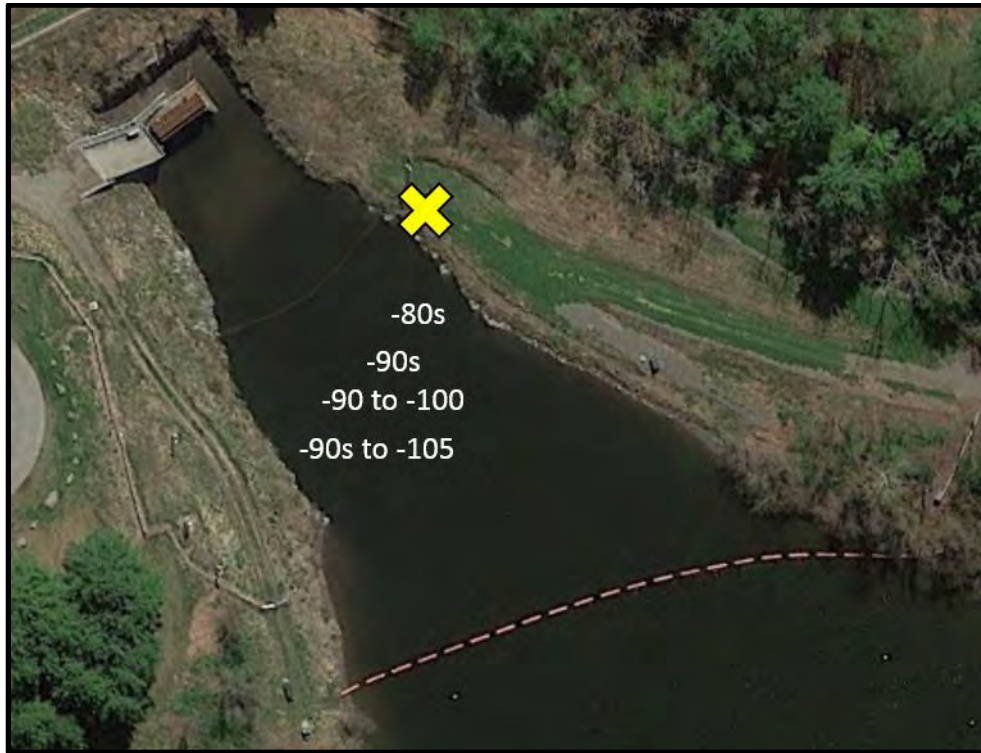
Figure 16: The large yellow X marks the approximate placement of the yagi antenna and the Orion receiver used to detect fish at the NMPS Intake at River Mile 127. The radio test tag produced power levels ranging from -80 to -105 with highest powers located closest to the yagi antennas and attenuated farther out from the antenna near the far bank of the intake.
