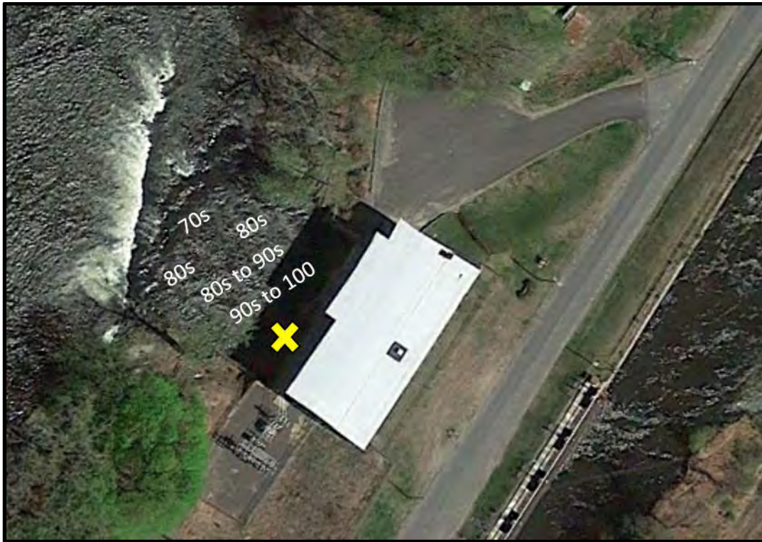
Figure 10: The large yellow X marks the approximate placement of the yagi antenna and the Lotek receiver used to detect fish within the Station No.1 tailrace at River Mile 121. The radio test tag produced power levels ranging from 70s to 100 with highest powers located closest to the yagi antennas and attenuating in the middle of the Station No. 1 Forebay.
