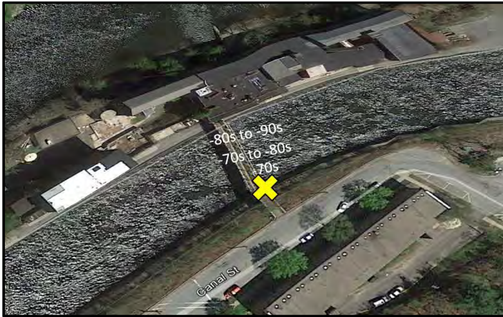
Figure 13: The large yellow X marks the approximate placement of the yagi antenna and the Orion receiver used to detect fish in the upstream end of the canal at River Mile 122. The radio test tag produced power levels ranging from -70 to -90s with highest powers located closest to the yagi antennas and attenuated farther out from the antenna.
