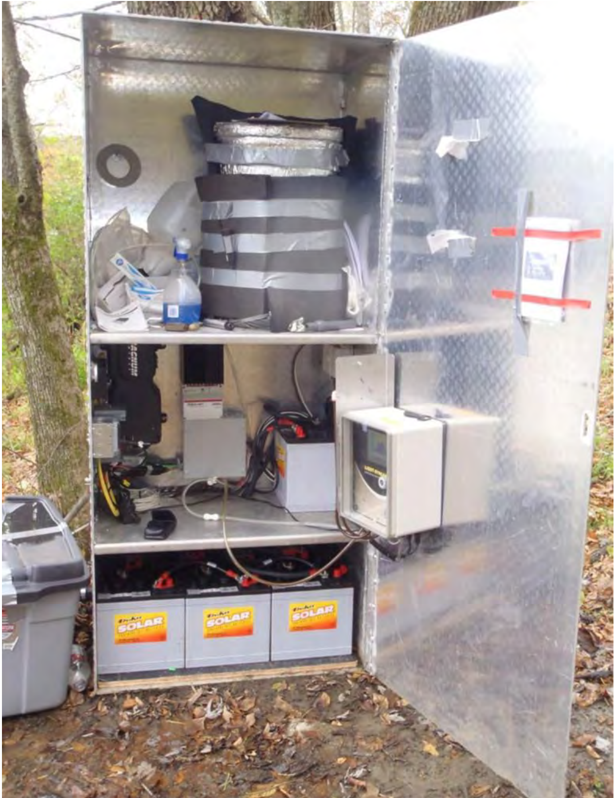
Figure 2.2.1-2 LISST StreamSide Equipment Cabinet Configuration
