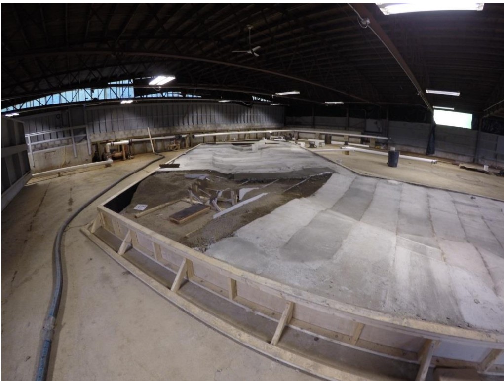
Figure 4-9: Model with mortar cap near the intake which remains to be installed.
