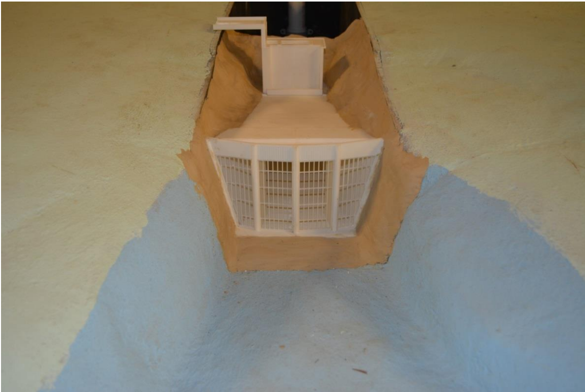
Figure 4-10: Modeled intake\discharge structure.
