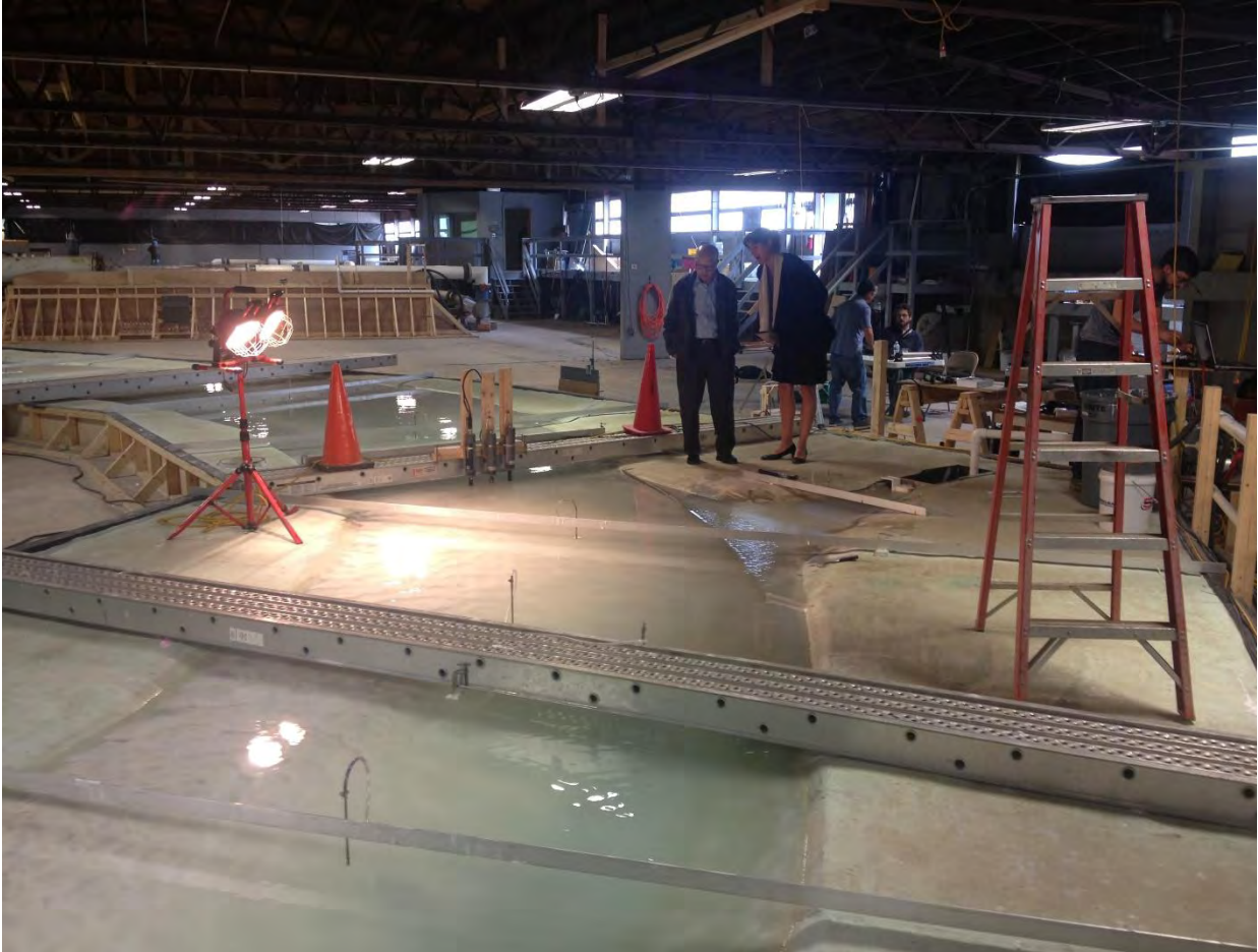
Figure 2.3.3-5 Physical Model of Northfield Tailrace Area- Bend in River is at the Tailrace
