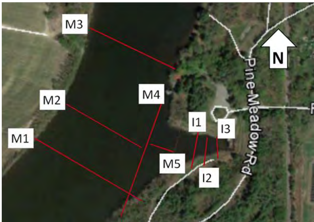
Figure 30: Velocity Transect Locations near Intake/Tailwater
