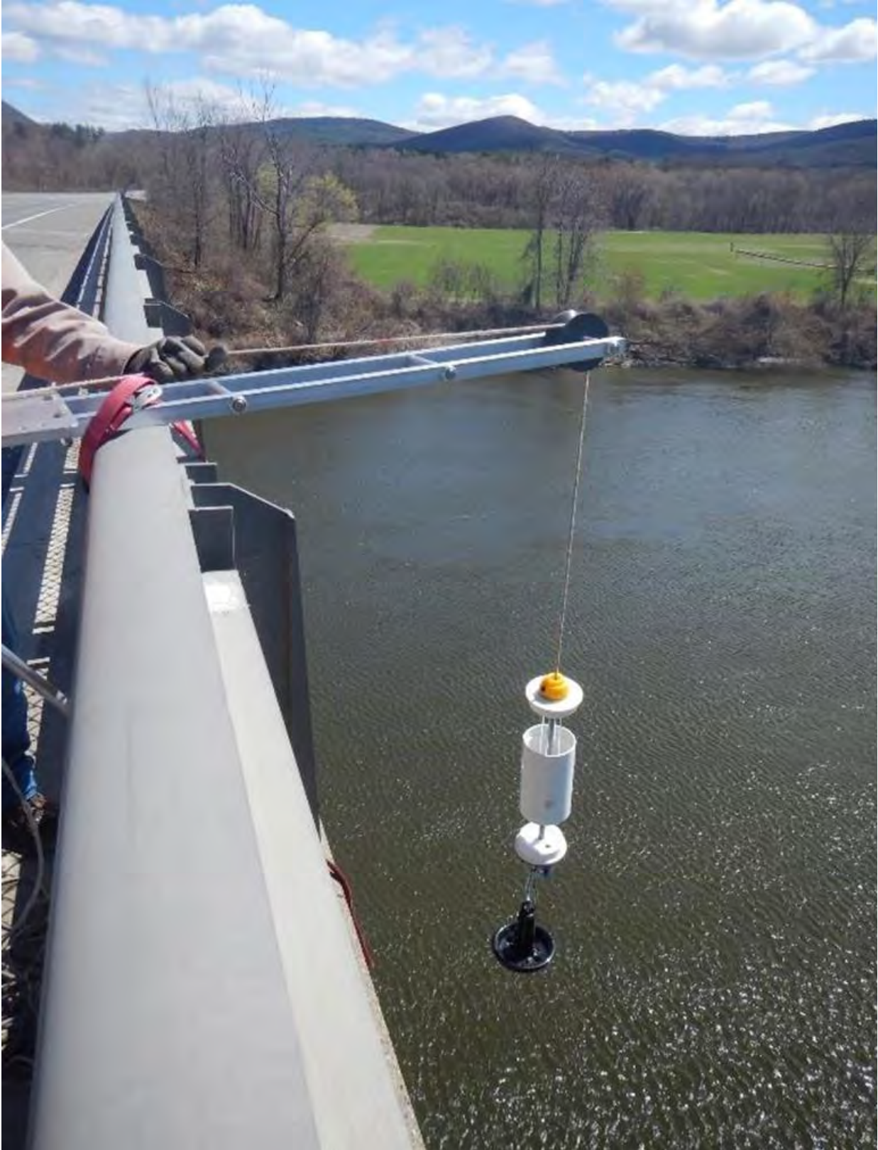
Figure 2.2.2-1 Configuration of Rt.10 Bridge Grab Sample Collection
