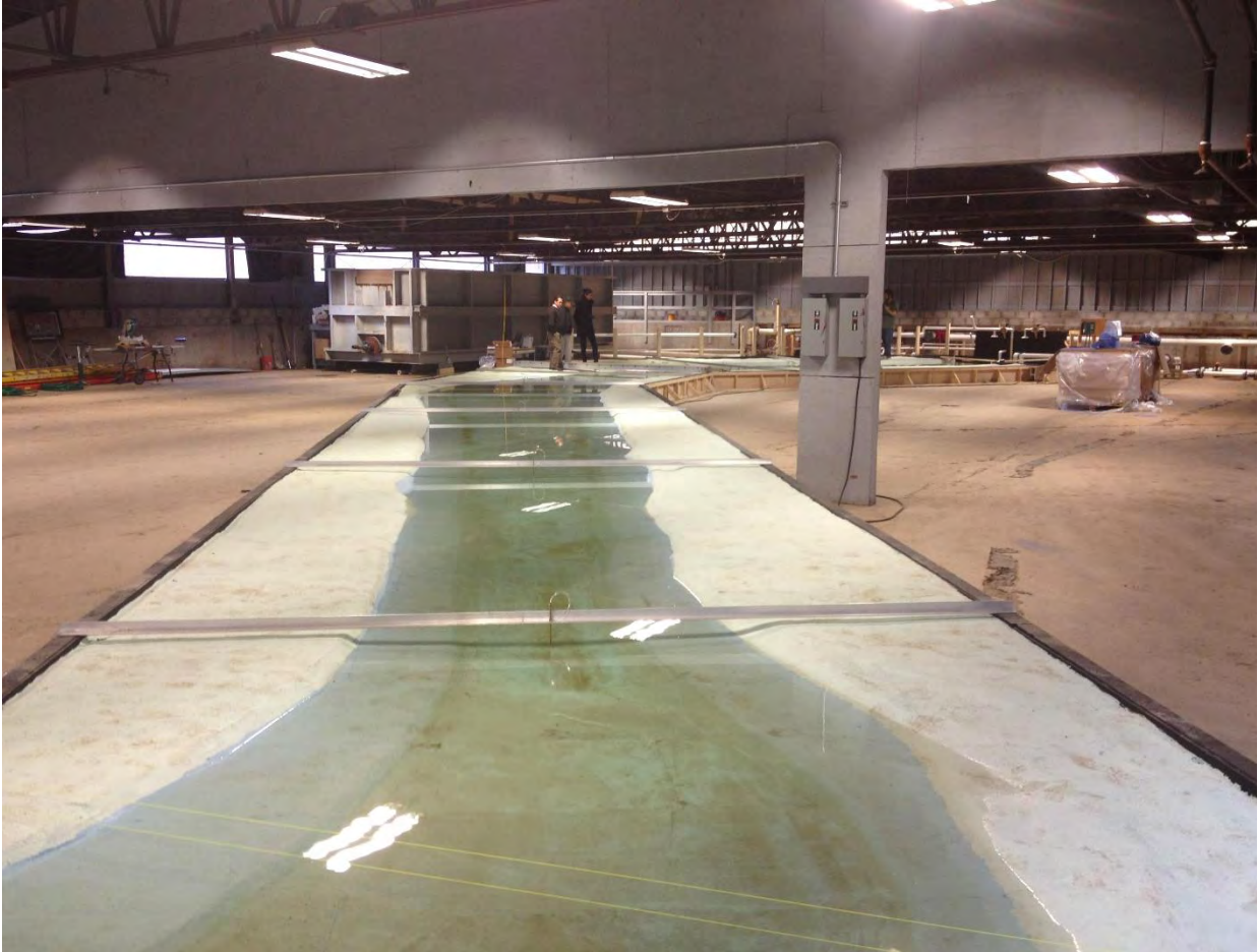
Figure 2.3.3-4 Physical Model of Turners Falls Impoundment - Northfield Tailrace Area
