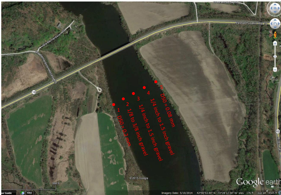
Figure 3-8: Location and D 50 of riverbed samples collected near Route 10 bridge.
