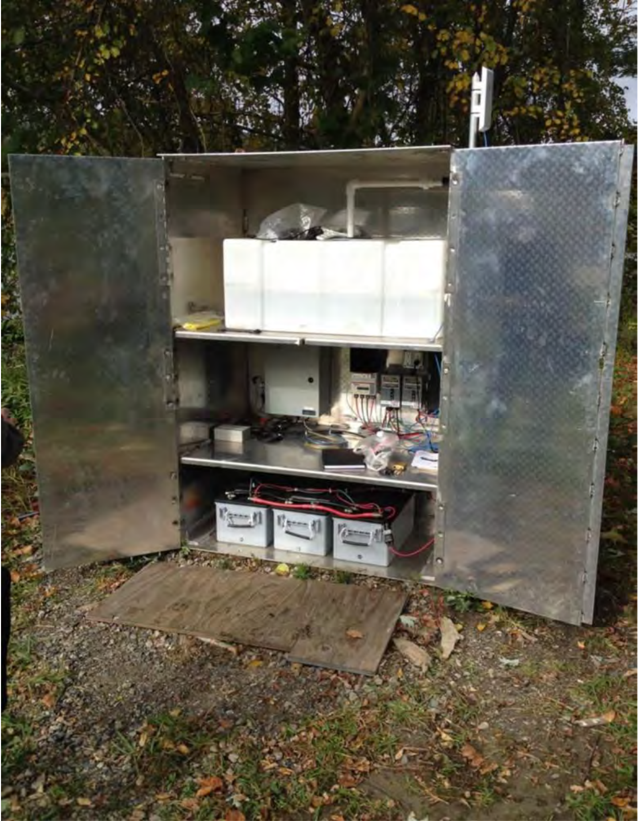
Figure 2.2.1-3 LISST-HYDRO Cabinet Configuration (typical)
