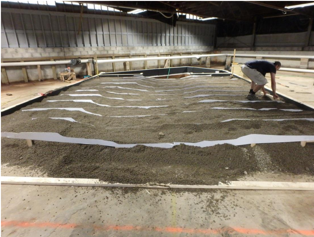
Figure 4-8: Model templates and spreading of fill material between templates.
