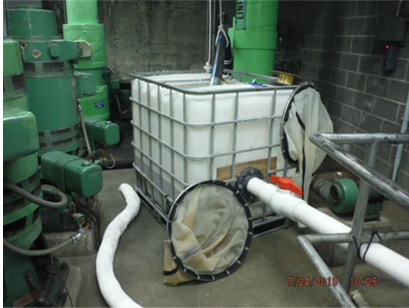
Figure 3.1-1: Ichthyoplankton Entrainment Collection Set Up for Collection of American Shad Eggs and Larvae at the Northfield Mountain Project, 2015
