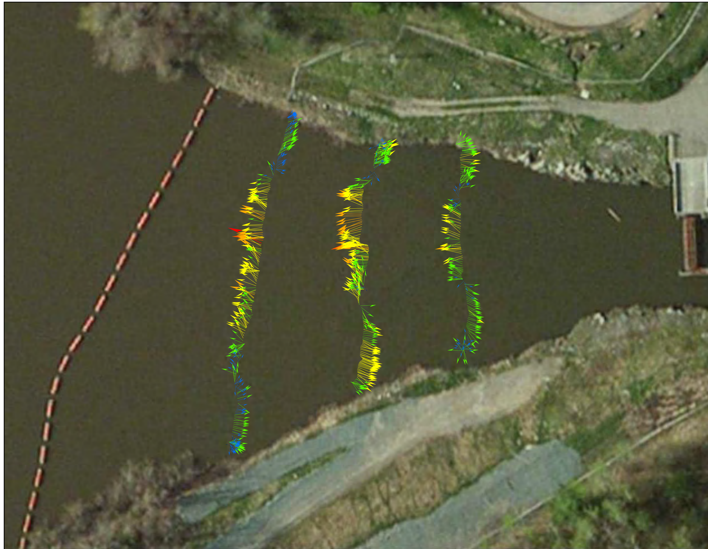
Figure 7.2-2 Depth-Averaged Channel Velocities at Transects below Northfield Tailrace (2 units at full hydraulic generating capacity ~10,000 cfs)
