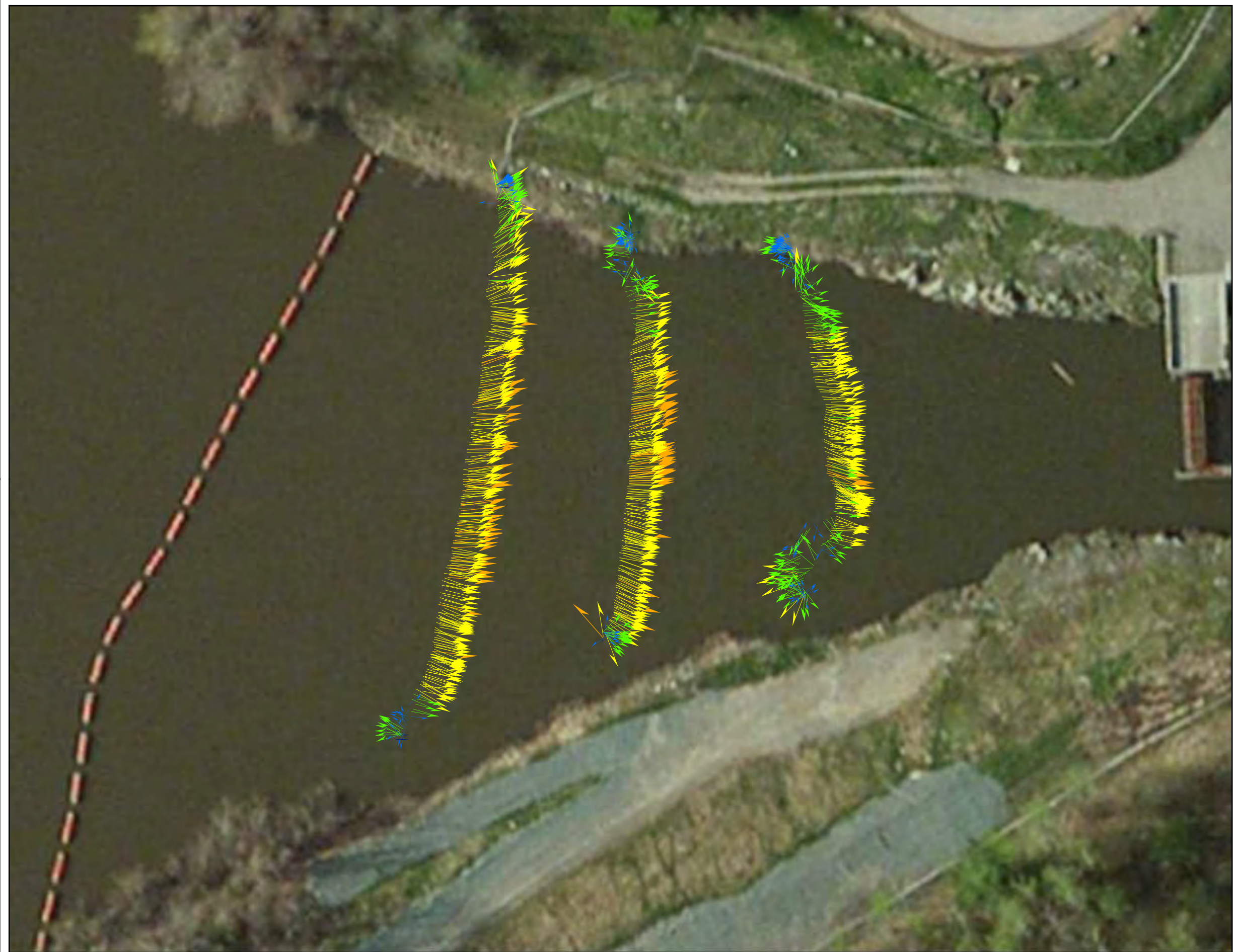
Figure 7.2-3 Depth-Averaged Channel Velocities at Transects below Northfield Tailrace (4 units at full hydraulic pumping capacity ~15,200 cfs)
