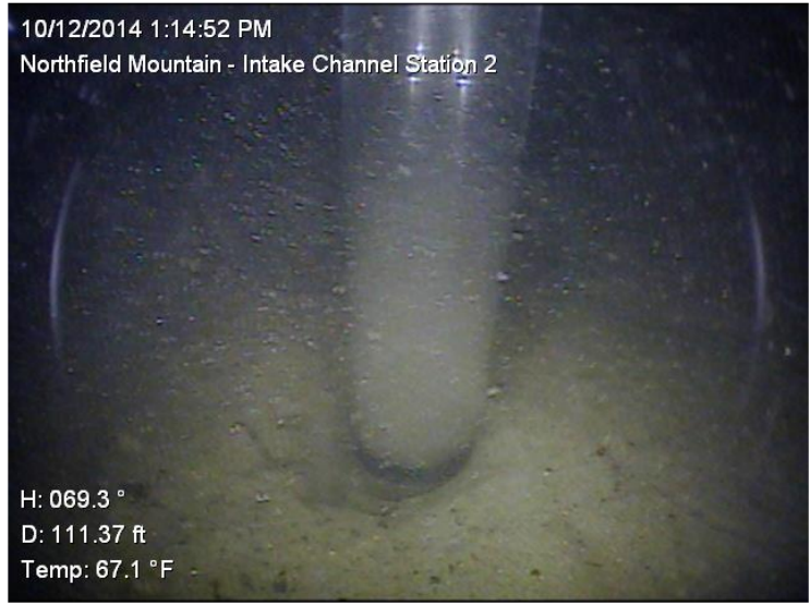
Figure 3.1-1 2014 Upper Reservoir Intake Channel Gravity Core Collection (2014)
