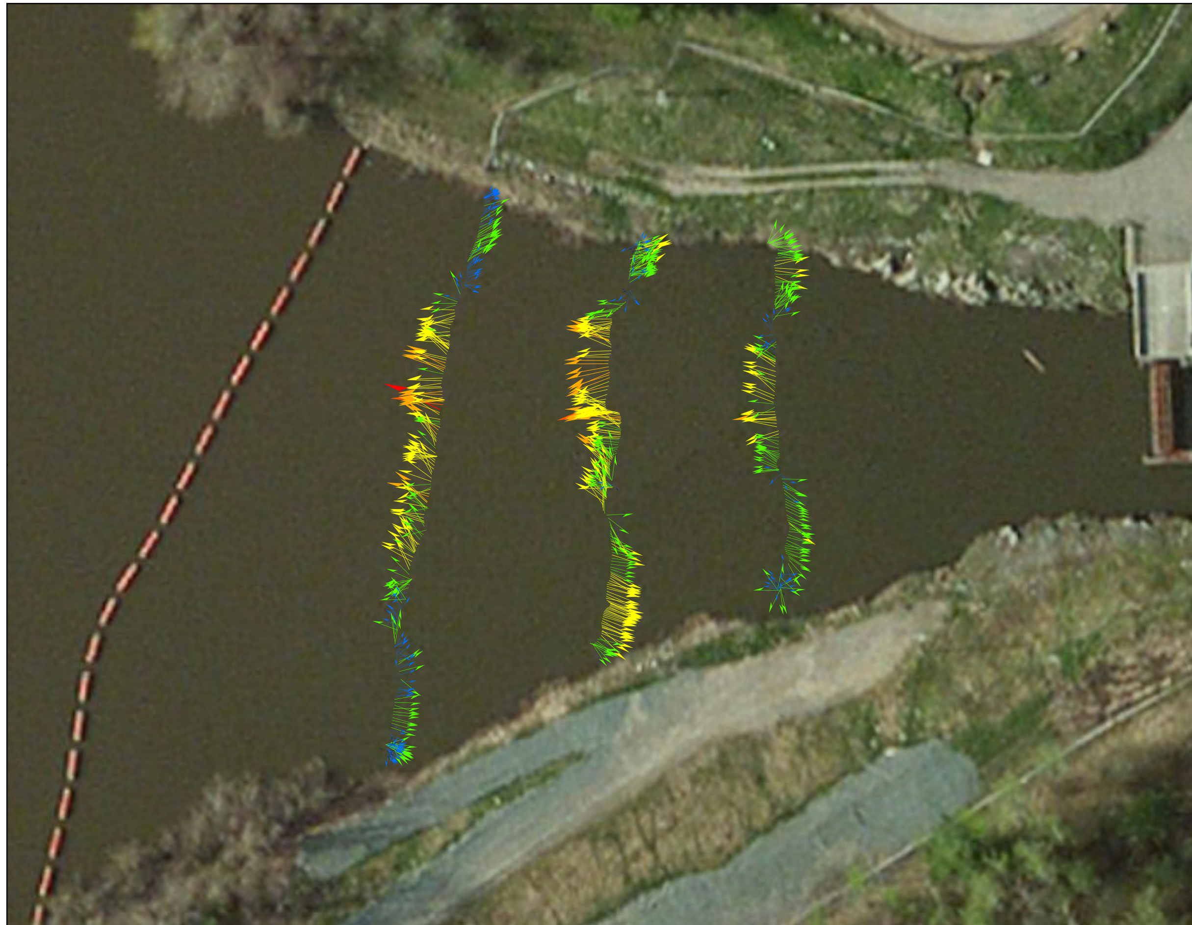
Figure 4 Observed Depth-Averaged Channel Velocities at Transects below Northfield tailrace (2 units at full hydraulic generating capacity ~10,000 cfs)
