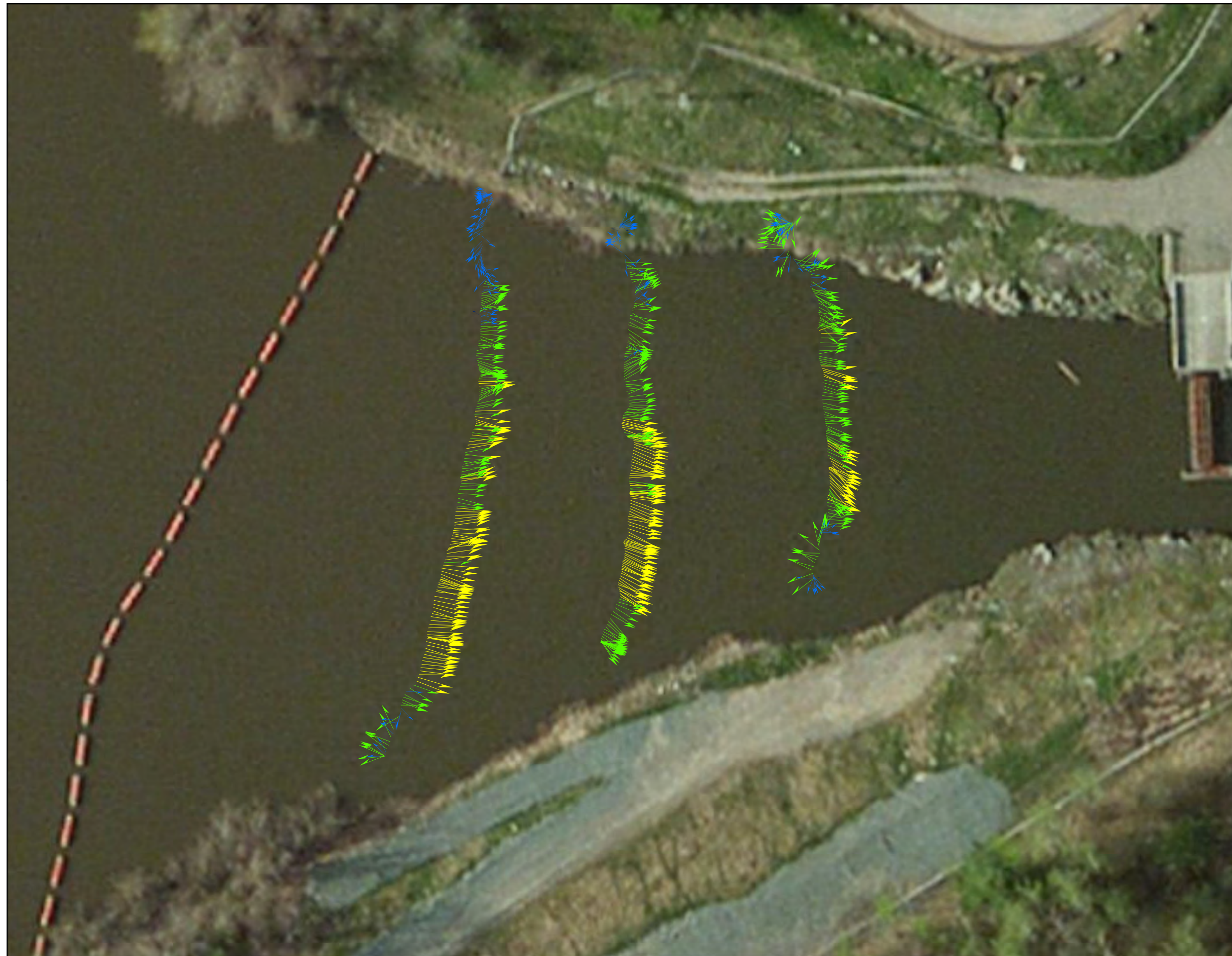
Figure 6 Observed Depth-Averaged Channel Velocities at Transects below Northfield tailrace (2 units at full hydraulic pumping capacity ~7,600 cfs)
