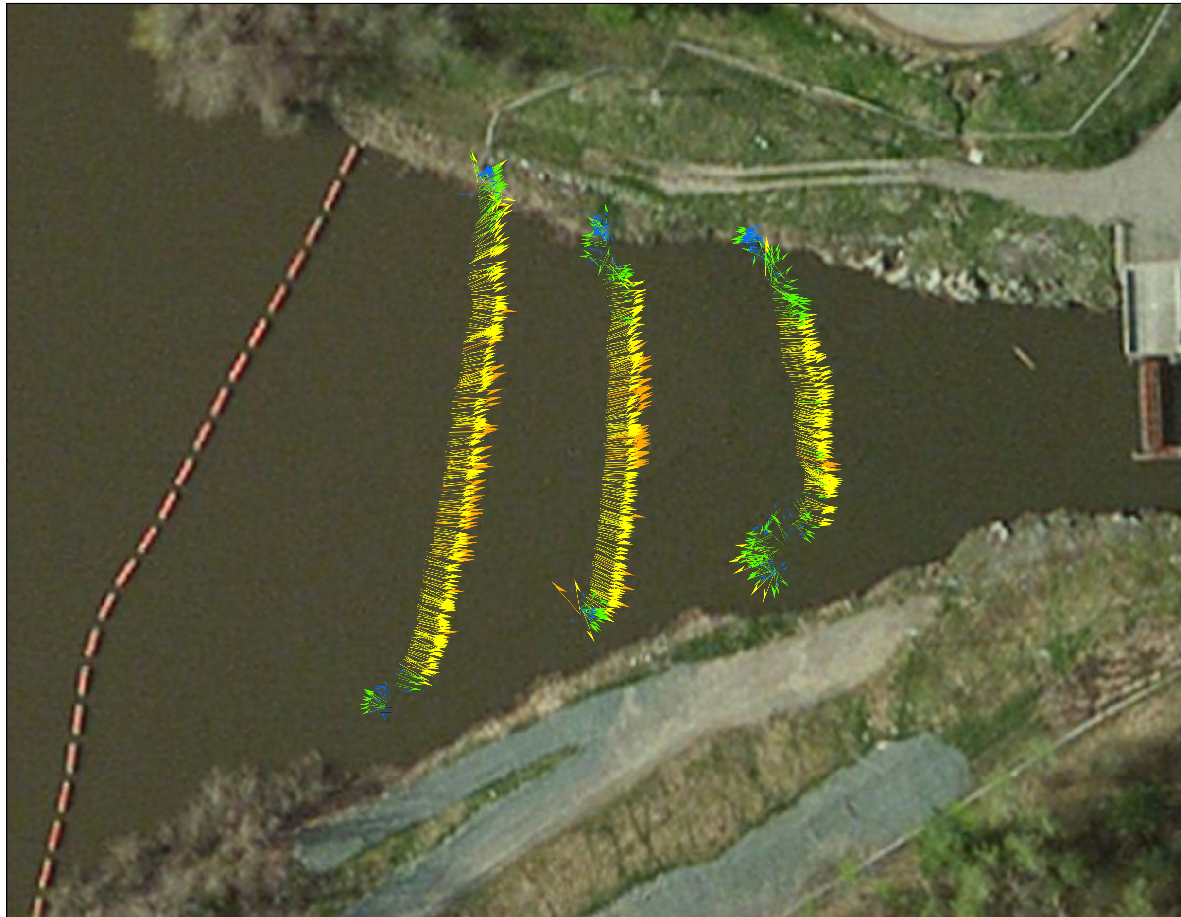
Figure 5 Observed Depth-Averaged Channel Velocities at Transects below Northfield tailrace (4 units at full hydraulic pumping capacity ~15,200 cfs)
