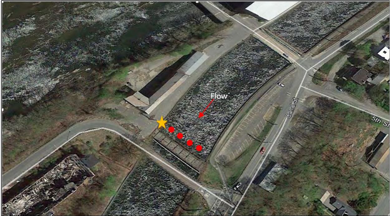
Figure 3. The location of the four split beam transducers (in red, not to scale) and a DIDSON (orange star, not to scale) used to monitor eel migration through the Turners Falls Project power canal, Turners Falls, MA.
