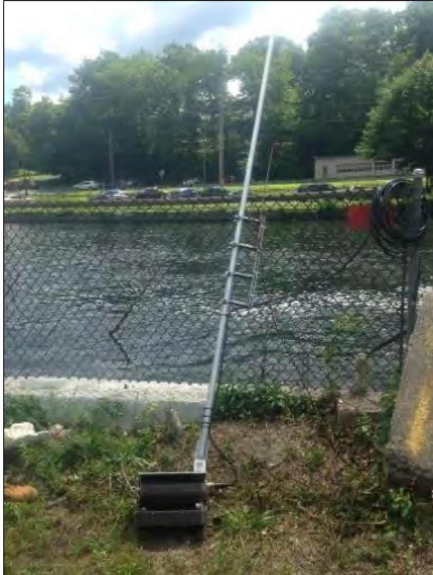
Figure 4. The DIDSON camera prepared for installation along the canal wall at the Turners Falls Project, Turners Falls MA.
