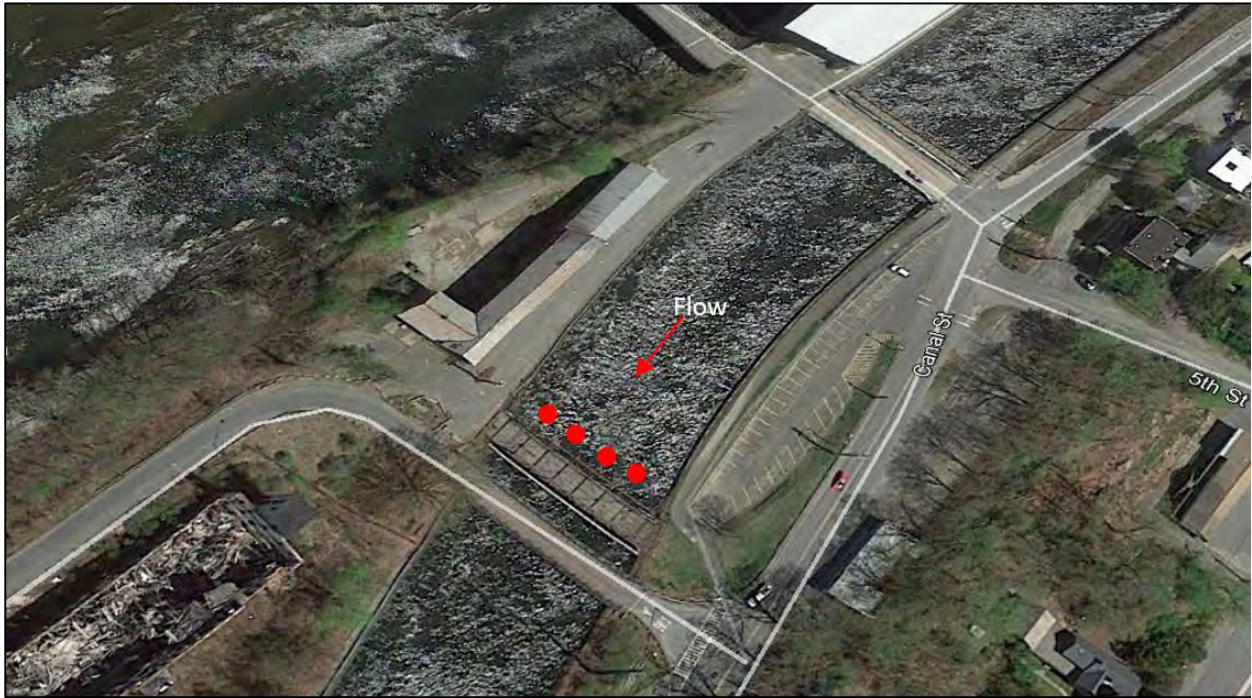
Figure 3. The location of the four split beam transducers (in red, not to scale) used to monitor juvenile shad as they migrate through the Turners Falls Project power canal, Turners Falls, MA.
