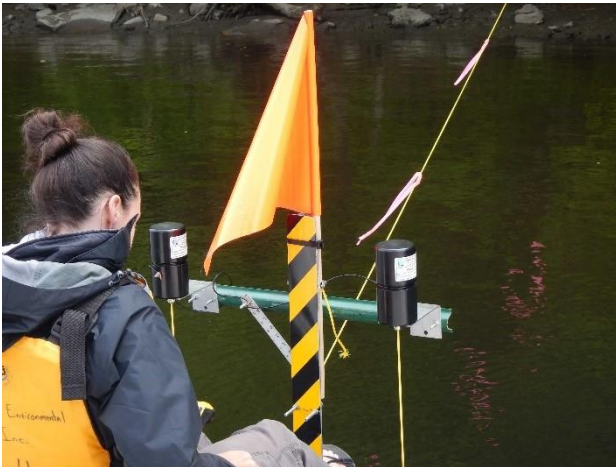
Clockwise from top: (1) digital image of a passing boat captured by the camera mounted to the Route 10 Bridge; (2) wave logger located just downstream of the Route 10 Bridge; and (3) Dual wave loggers located just upstream of the French King Bridge
