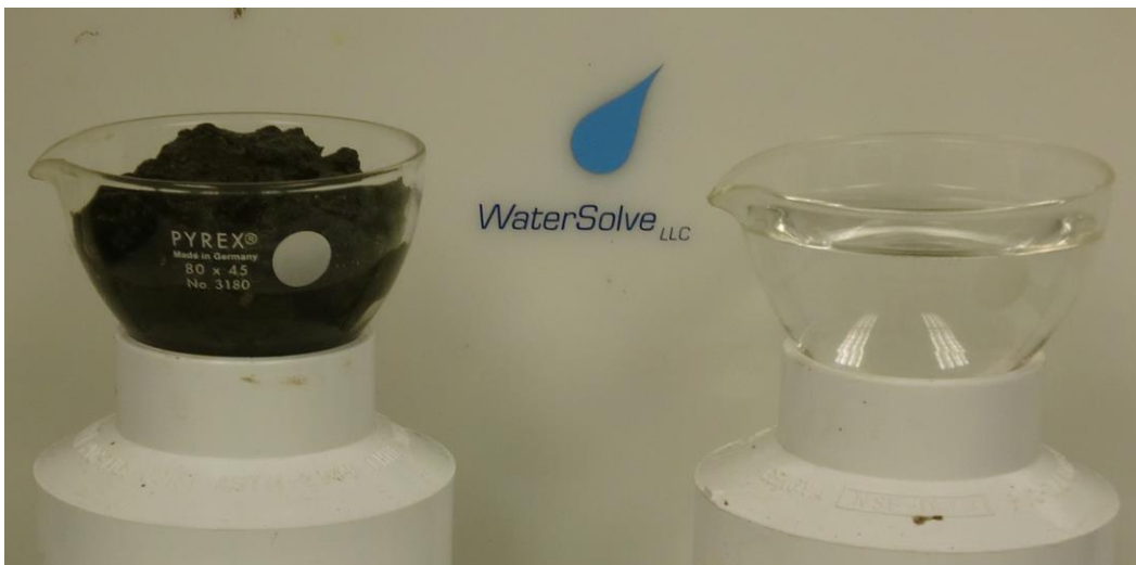
One thousand milliliters of diluted and conditioned sediment sample was dewatered using Geotube® GT500D fabric. The captured solids and filtrate are shown above.
