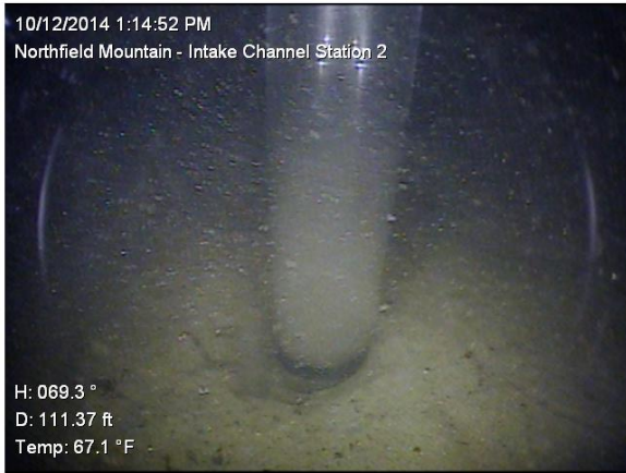
Figure 2.1: Gravity core sample depicting the barrel penetrating into sediment.
