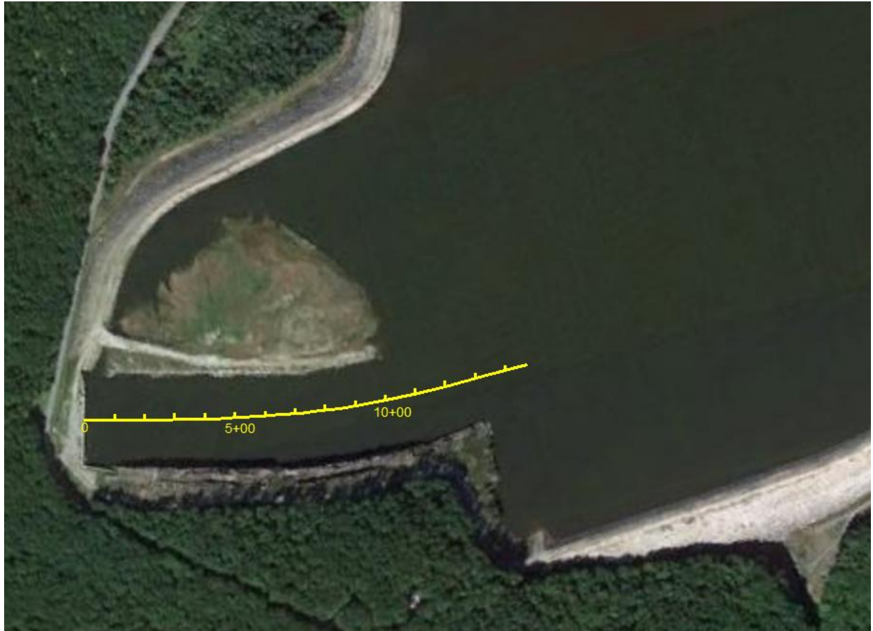
Figure 40. Intake Channel Station Line
