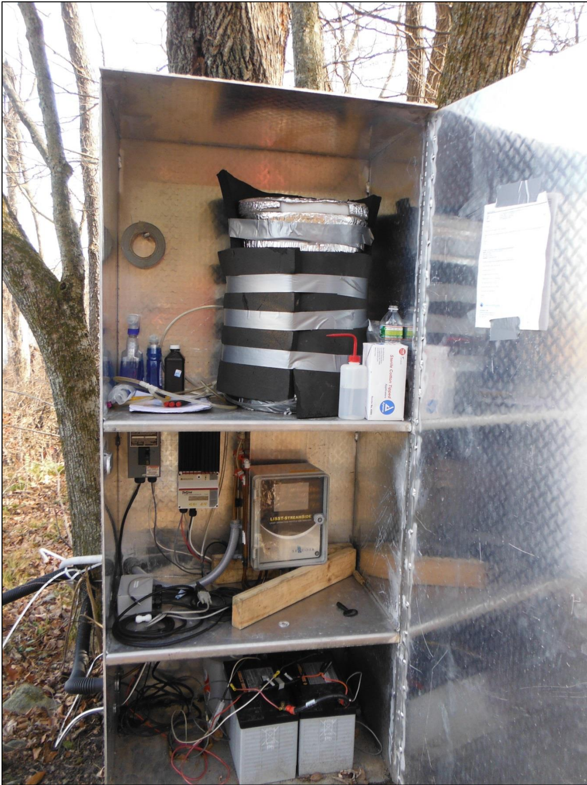
Figure 3.2: Configuration of the LISST StreamSide. The batteries were charged using solar panels.
