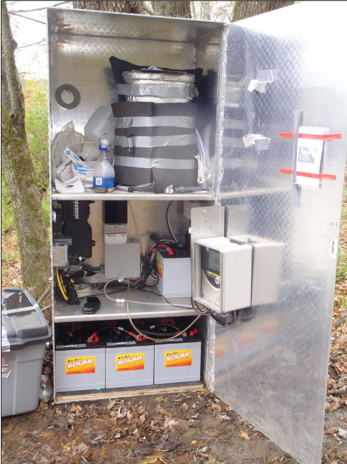
Figure 3.3: Configuration of the LISST StreamSide from October 23, 2014 to present. The batteries are charged using solar panels.
