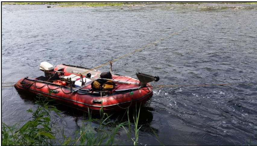
Photo 2. Raft and stationing rig used for bed profile and water velocity data collection in unwadable areas.
