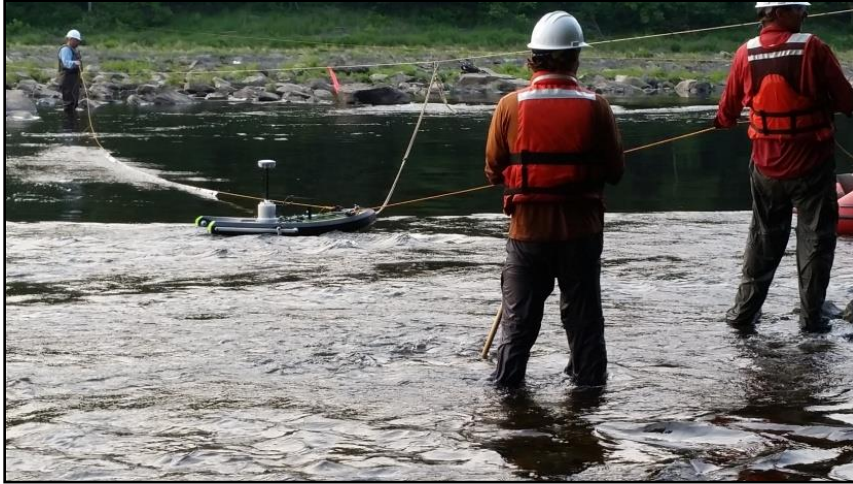
Photo 3. Velocity data collection with an ADCP unit.
