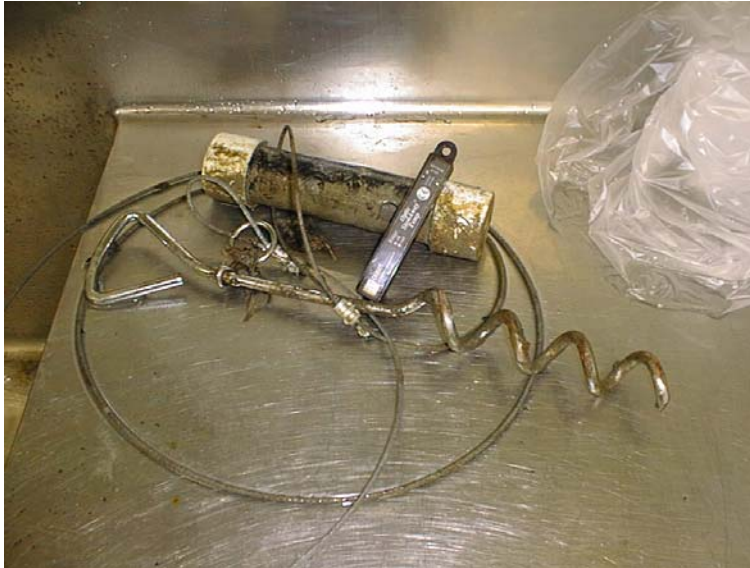
Stowaway sensor, plastic tube and cable (anchor screw optional; unit assemblies typically cabled to fixed object, e.g., large tree)
