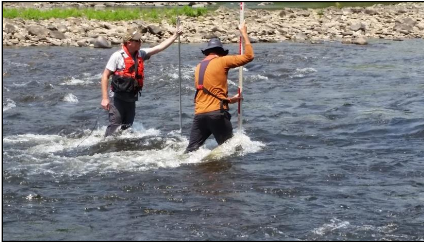
Photo 1. Bed profile and water velocity data collection on a wadable transect at low flow.
