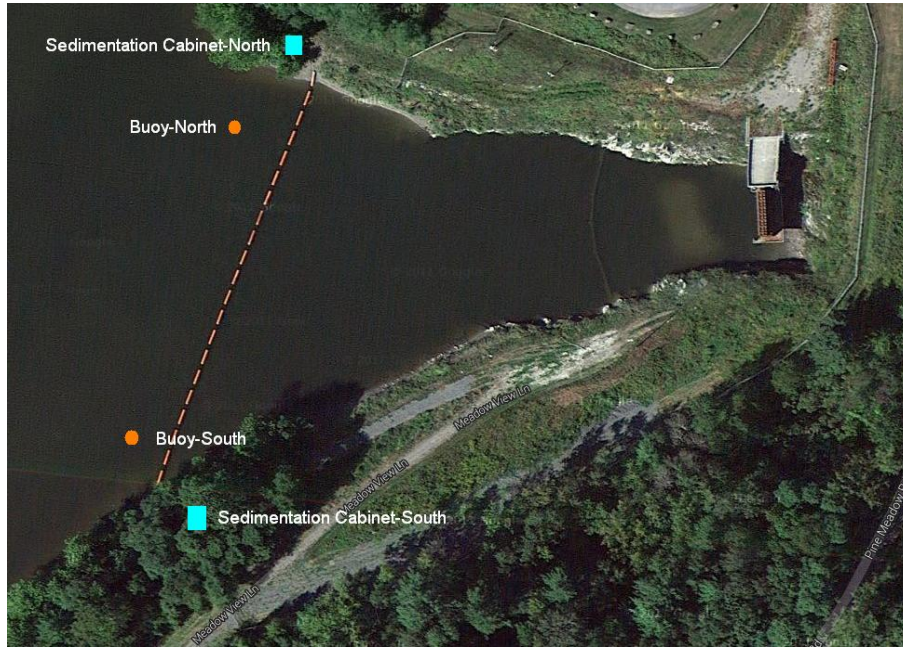
Aerial Photo depicting LISST-HYDRO configuration at Tailrace
