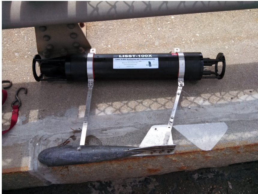
LISST-100X and weighted fin used for stability at Route 10 Bridge
